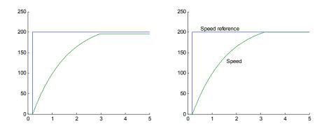
Solution: Left is with P-controller since there is a stationary speed error.
