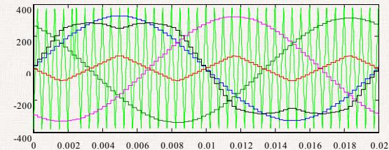
Maximum phase voltage with sinusoidal modulation :  $U_{dc}/2$
