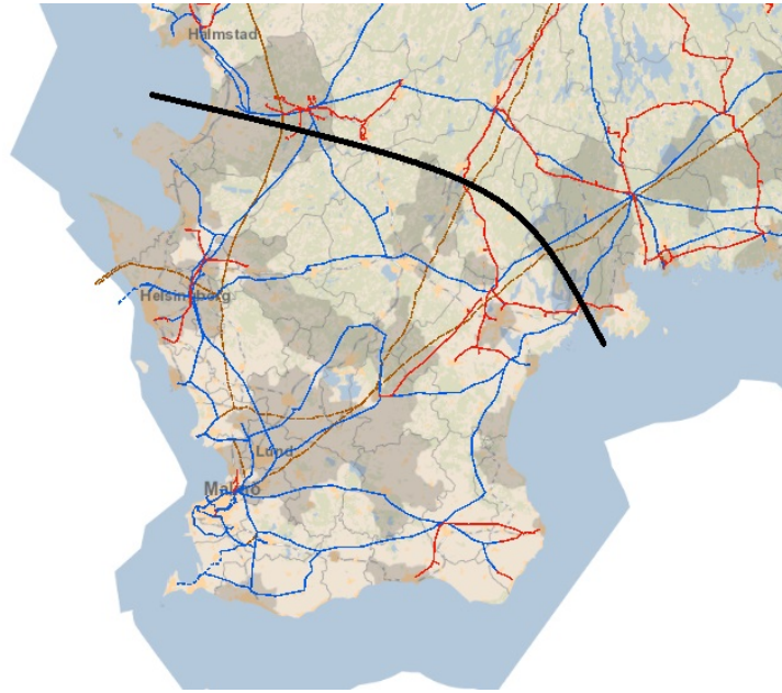
Figure 3.6: Map showing the sub-transmission grid in the study area, where brown lines represent transmission lines (400 kV), blue lines represent sub-transmission lines (135 kV), and red lines represent 50 kV lines. The black line indicates the approximate border of the Skåne region. Image from E.ON Sweden.
