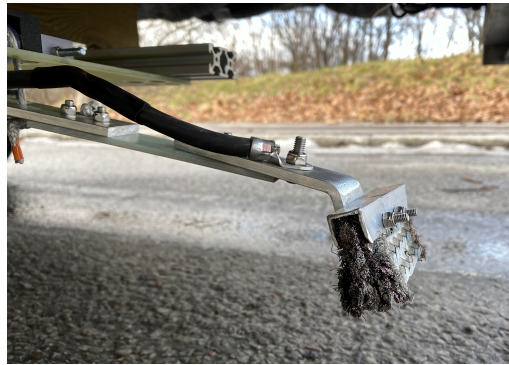
Figure 3.22: The sliding contact in the trailer. Figure taken from [44].
