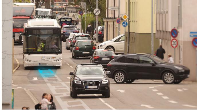
Figure 1.3: A bus line in Balingen, Germany where Electreon's wireless charging technology is implemented.[24].
