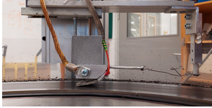
Figure 3.8: One of the two sliding contacts in the RTR. The sliding contact mount is attached to a horizontal sliding bearing and connected to a load cell via a steel wire, enabling the measurement of the friction force.
