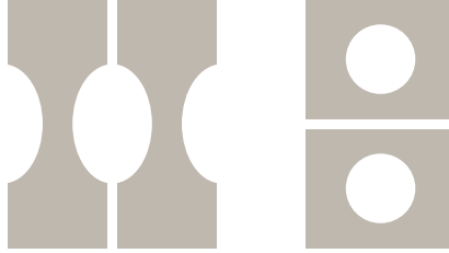
Figure 1.3: Left: Cross section of two rectangular winding with concave indents along the sides. Right: Cross section of two rectangular hollow windings with inner circular coolant channels.
