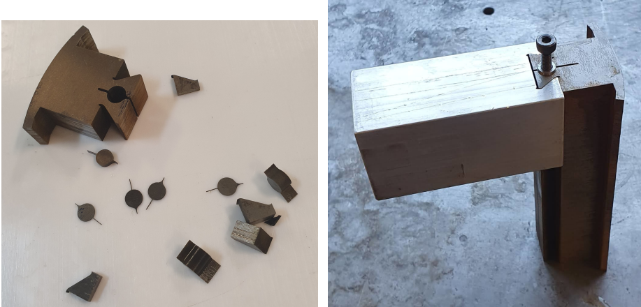
Figure 5.5: Left: Photo of the first test of electric discharge machining of shorter tooth sample. Right: Photo of the first electric discharge machined tooth of full length, fit into a test sample of a mortise joint in aluminium.
