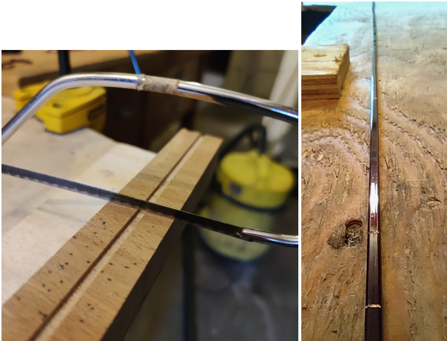
Figure 3.26: Left: Rig for hacksawing a straight conductor. The groove is 2.3 mm deep so that 0.7 mm of a conductor protrudes above the surface of the rig. Hacksawing down to the surface will thus result in a 0.7 mm deep cut. Right: A straight conductor 2 m conductor with 22 cuts made with the hacksaw, ready to be bent.
