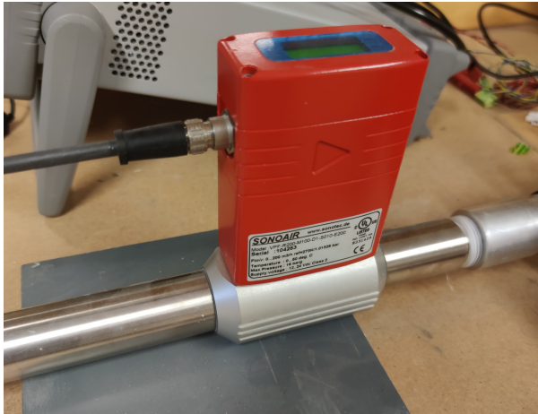
Figure 6.4: Photo of the Sonoair VPF R200 flow meter used to measure the airflow rate.
