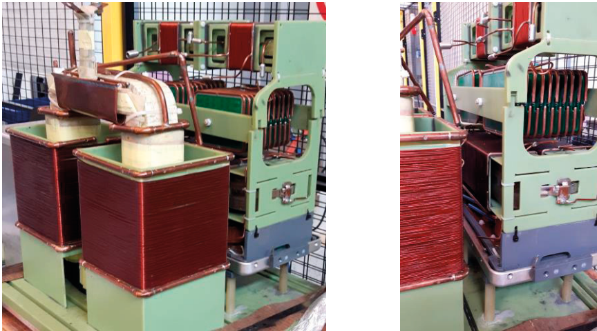
Figure 8.11: Overview of early prototype high-voltage module (enclosure removed for clarity)
