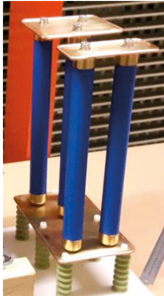
Figure 4.142: Resistive load used in testing the developed split-core pulse transformer
