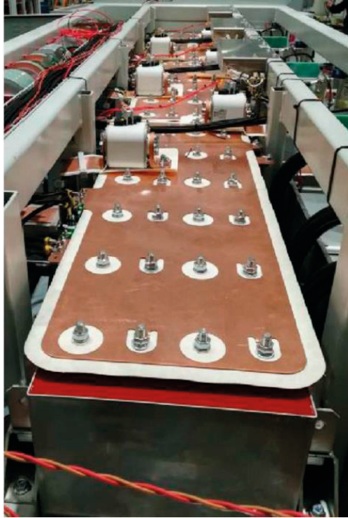
Figure 9.70: Top-down view of complete full-scale modulator exposing row of capacitors comprising the main capacitor bank. The roof has been removed for clarity.
