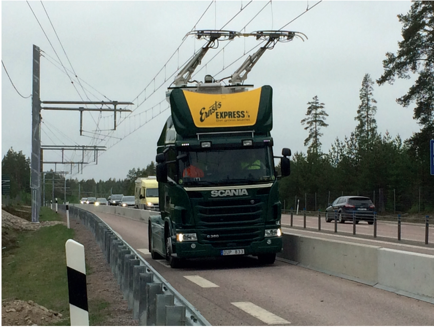
Figure 1.6: One of the test sites of road bound conductive ERS on public roads in Sweden. Photo: Region Gävleborg
