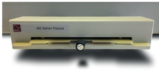
Figure 3.2: This fixture features four contact plates providing true four wire impedance measurement. A cylindrical capacitor is the DUT in this example. Valid frequency range for this this method is DC-35MHz. NB! A frequency is always needed for the LCR measurements and DC shall here be interpreted as 10μHz.
