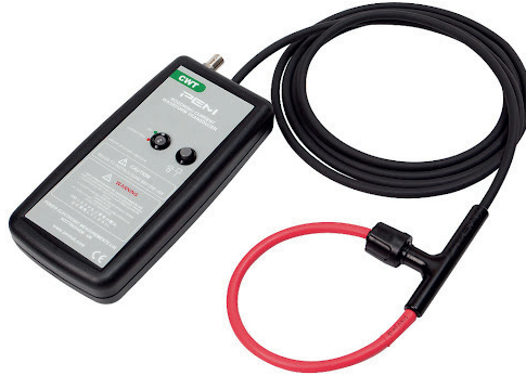
Figure 5.4: PEMUK CWT Rogowski coil. Picture from PEMUK
