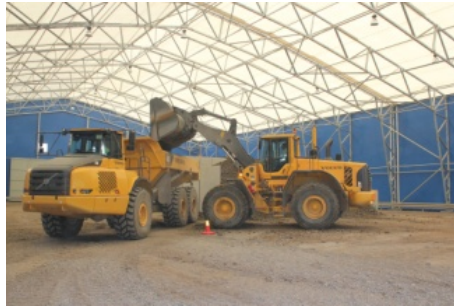
Fig. 2.1 Measurement setup for the “short loading cycle gravel”.
