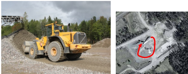
Fig. 2.2 Measurement setup for the “load and carry gravel”. Left; the gravel pile during the bucket fill phase. Right; aerial view of the route from the gravel pile to the hopper.
