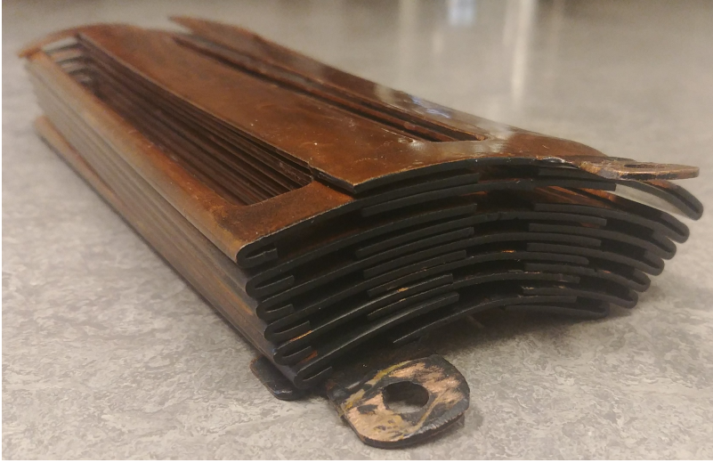
Figure 3.6: Example of folded laminated windings for a machine with long active length.
