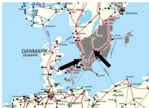
Fig. 2: Blacked out area (gray area) for 2003 Swedish/Danish blackout, also the substations where reactor hunting happened.
