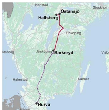
Fig. 1: The South-West link ongoing project in Sweden, the northern part is an AC connection from Hallsberg substation to Barkeryd substation and the southern part is a DC connection from Barkeryd substation to Hurva substation [15].
