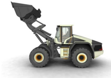
Fig. 6.3 Wheel loader with in-wheel drive traction electrical machines
