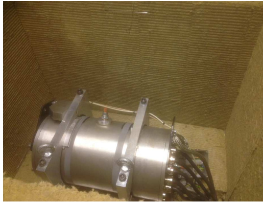
Fig. 6.13 EM3 placed inside a temperature insulated chamber [107]
