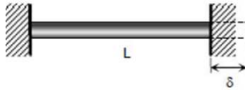
Fig. 4.1 Bar with both ends fixed [75]
