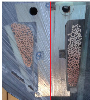
Fig. 6.8 Cross section of the 1 st group (left side) and 2 nd group (right side) of the designed and produced test motorettes
