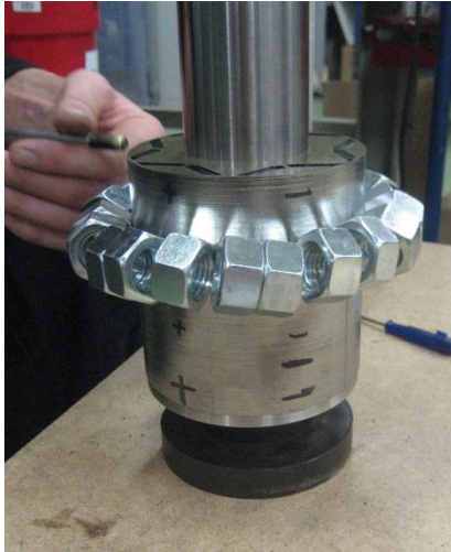
Figure 4.8 Rotor magnets insertion with a crown of iron pieces (nuts) keeping the magnets and checking the polarity of the magnets
