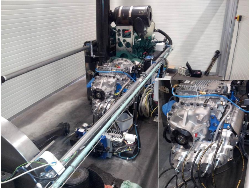
Figure 5.18 Test facility for the system testing with the gearbox, gear drive and electric machine focused in the inset picture
