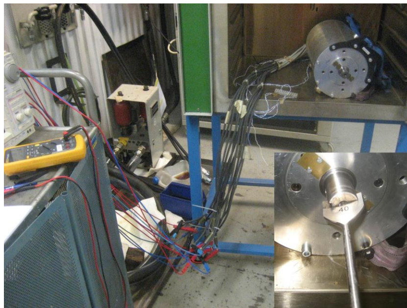
Figure 5.5 Test set up for temperature dependence measurements with the custom made fork connected to the shaft in the small picture
