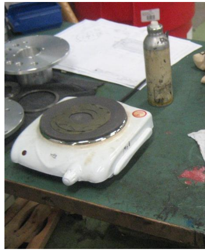
Figure 4.7 Rotor laminations pre heated on a stove before shrink fitted onto the rotor shaft
