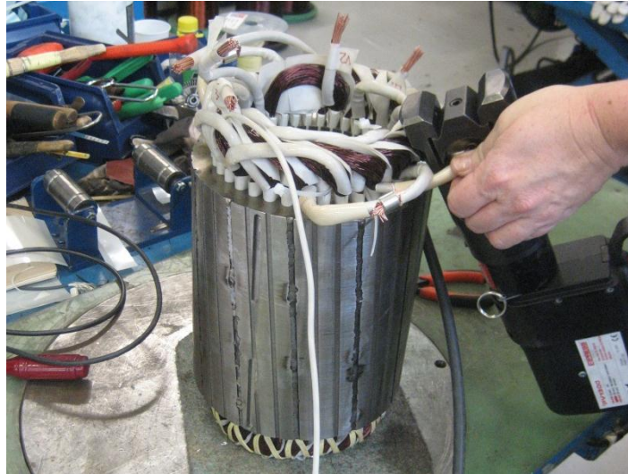
Figure 4.3 Clamping of the end windings
