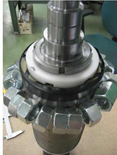
Figure 4.9 Rotor assembly being prepared for epoxy filling
