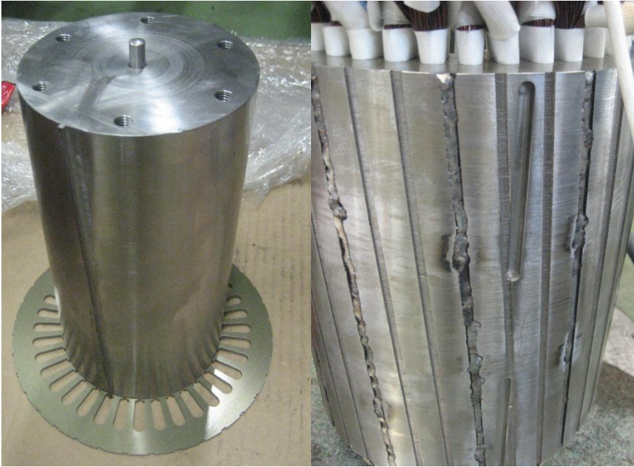
Figure 4.1 Stator lamination stacking at the manufacturing tool
