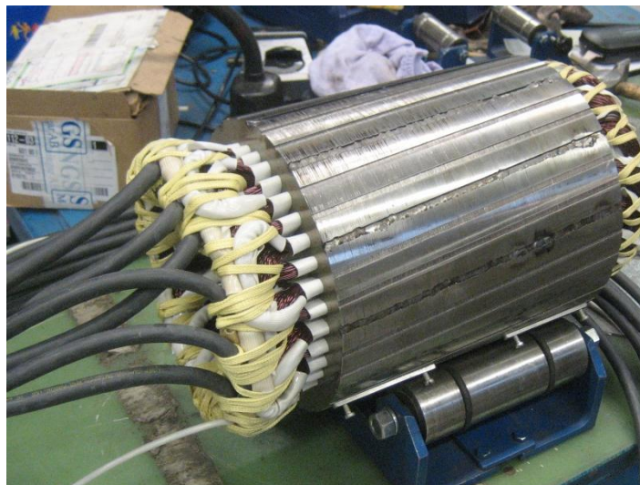
Figure 4.4 The completed active stator with three phase connection cables and three connection cables for the neutral point
