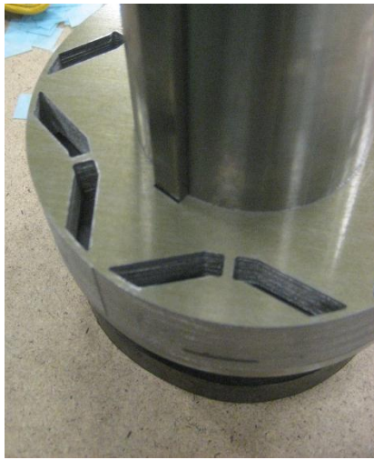
Figure 4.6 Rotor lamination stacking at the manufacturing tool using the wedge as guide
