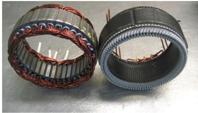
Figure 2.2 Conventional round wire winding (left) compare to hairpin winding (right)
