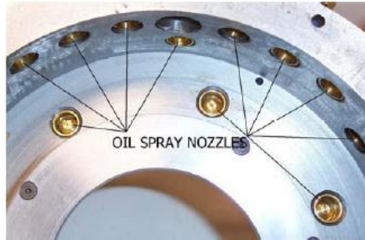
Figure 2.6 Spray nozzle locations inside motor housing [20]
