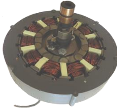
Figure 5.22 The prototype rotor assembled together with a stator segment.
