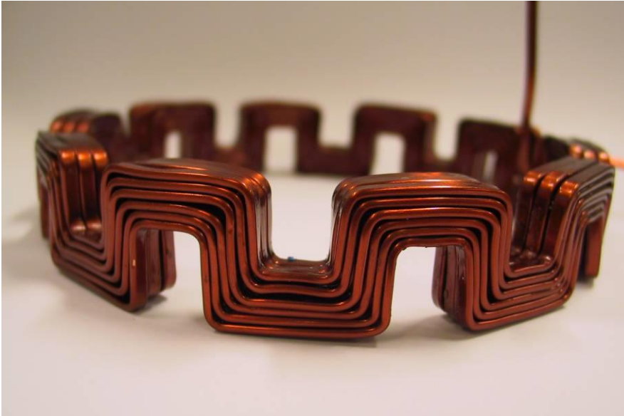
Figure 5.18 A handmade winding with a square conductor (to increase the copper fill factor) and 18 turns.
