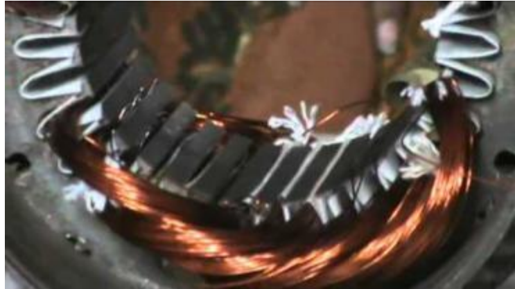
Figure 3.2 Distributed overlapping winding placed in a stator. Here, the stator acts as a bobbin.
