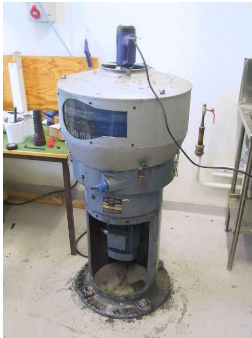
Figure 2.5 Rotocast rig with a thermal device on top.
