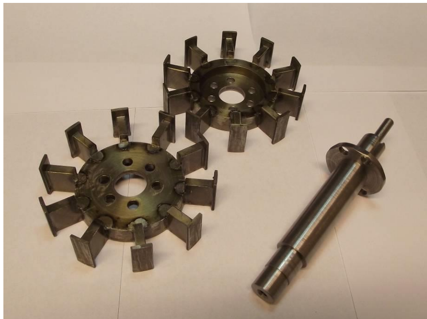
Figure 5.21 The prototype rotor, disassembled.
