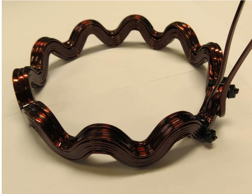
Figure 5.19 A fixture-pressed sinusoidal wave winding with 18 turns.
