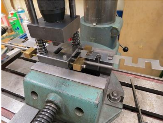
Figure 7.4 Cutting the second side to finish the strip before using it to form a winding.
