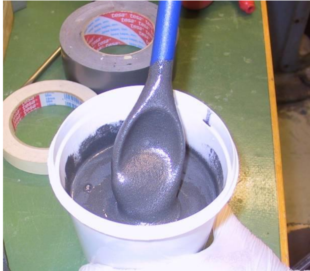
Figure 2.2 SMC and binder are mixed together to create SM 2 C for moulding.
