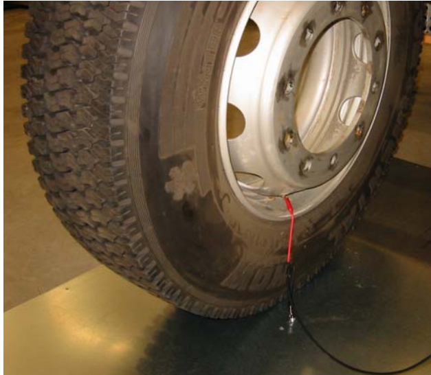
Figure 2.17. Measurement setup for determining the capacitance between one wheel and ground.
