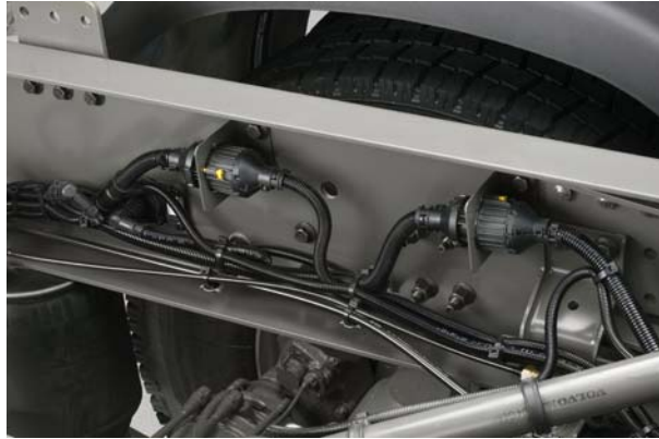
Figure 5.2. Frame rail and conductor layout. Picture from [76].
