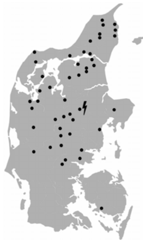
Figure 1.2 Eltra service area. 47 local CHP units, larger than 2 MW each, with a production of 347 MW were tripped. It is unknown how many units smaller than 2 MW that were tipped.
