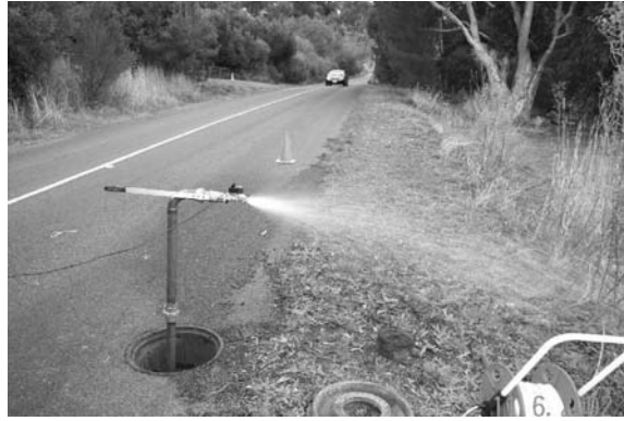
Figure A.8: Experimental burst
