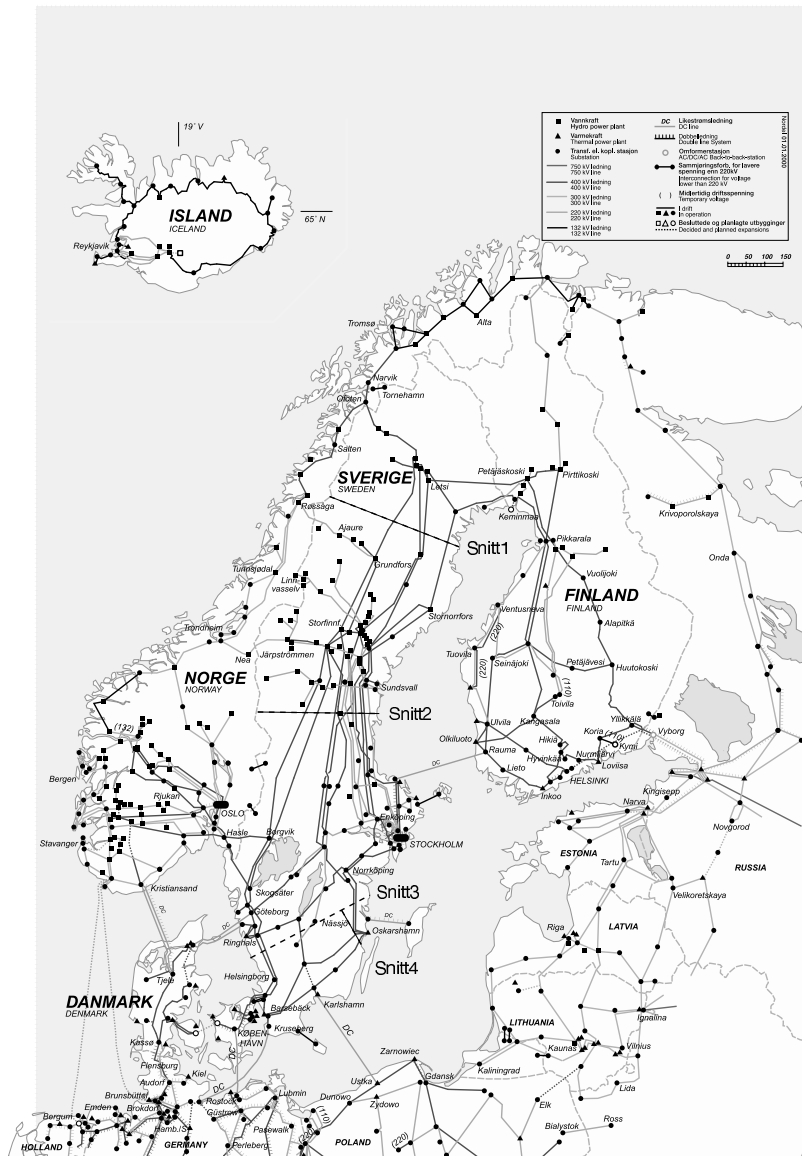
Figure 3.1: The NORDEL main grid, 2000. The cut-sets, Snitt 1 to 4, are marked.
