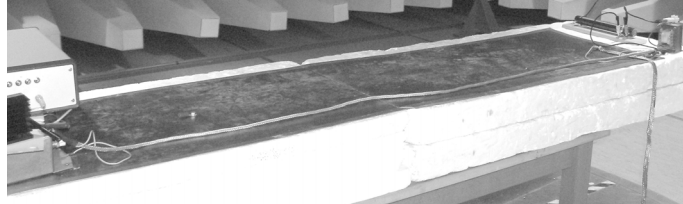
Figure 7.10. A picture of the set-up when shielded cables are used between the converter and the load.
