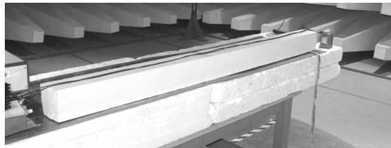
Figure 7.17. Both cables between the converter and the load are raised 11 cm above the ground plane. The cables are placed next to each other.
