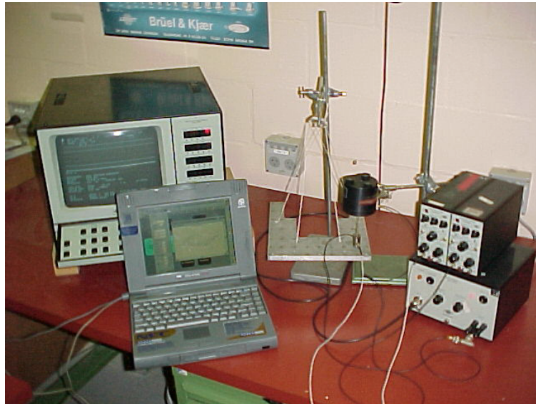
Figure A.4: Laboratory set-up for the free response analysis of the plate.
