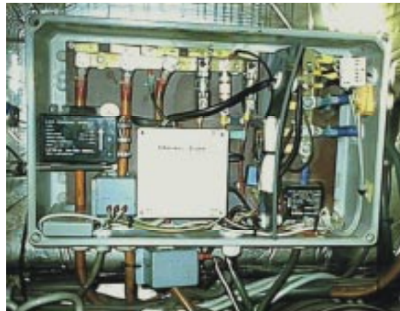
Figure 5.3: The current transducers around the cables in the power connecting points in the busses. At the top the “PTB”-box in the Neoplan bus and at the bottom “Grundbulten” in the Scania bus.
