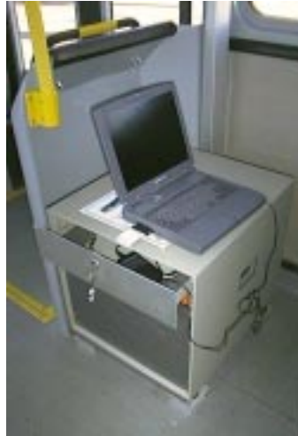
Figure 5.1: The computer and measuring system assembled in the Neoplan bus.
