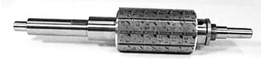
Figure 5.12 The rotor, with the magnets mounted but without the retaining layer of kevlar.
