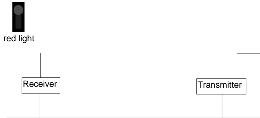
Figure 2-3. A track circuit with the transmitter disconnected.
