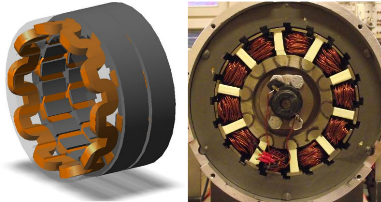
Figure 2.20 Stator core consisting of 3 axially distributed segments (left) and single phase prototype machine where different stator core prototypes were tested (right) [31]
