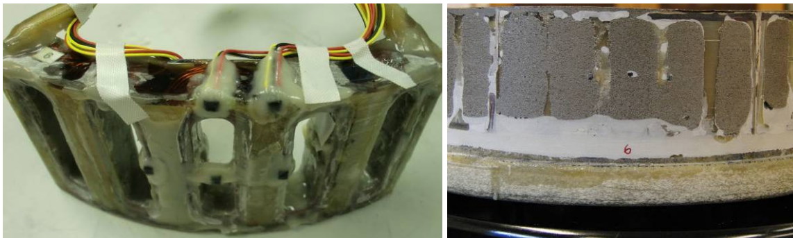
Figure 2.12 Inclusion of hall sensors (left) and their location after molding and machining (right)
