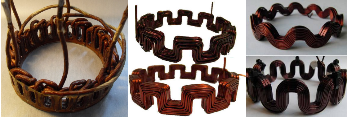
Figure 2.11 pre-formed coils: 22P24S distributed concentrated winding (left [14]) and wave windings (middle [19] and right [25])
