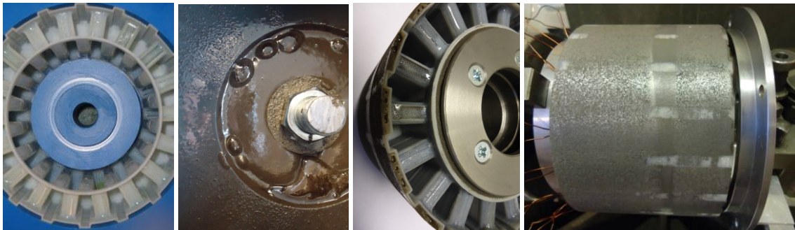
Figure 2.18 The mold with the main insulation system (left), the exchange process (left from the middle) and the ready stator from top and side view [34]
