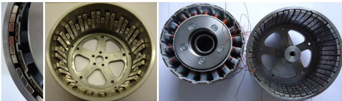
Figure 2.19 Air-gap between rotor and the stator, mounting process of permanent magnets and machine parts in prior to stator core evaluation [34]
