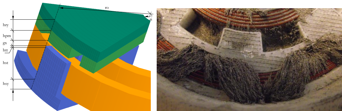
Figure 2.4 Parameterized machine (left) and bottom view of the machine where the iron powder flux paths that are defined by PM excitation are shown.
