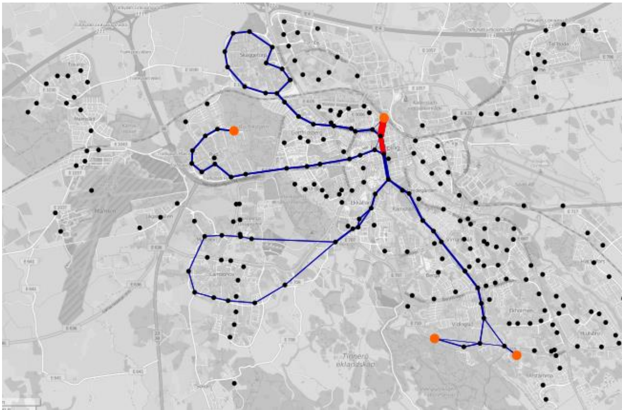
Figure 9 A map of bus line 1, 2, 3 and 4. Red lines show electric roads. Orange dots show charging stations. Black dots show bus stops.
