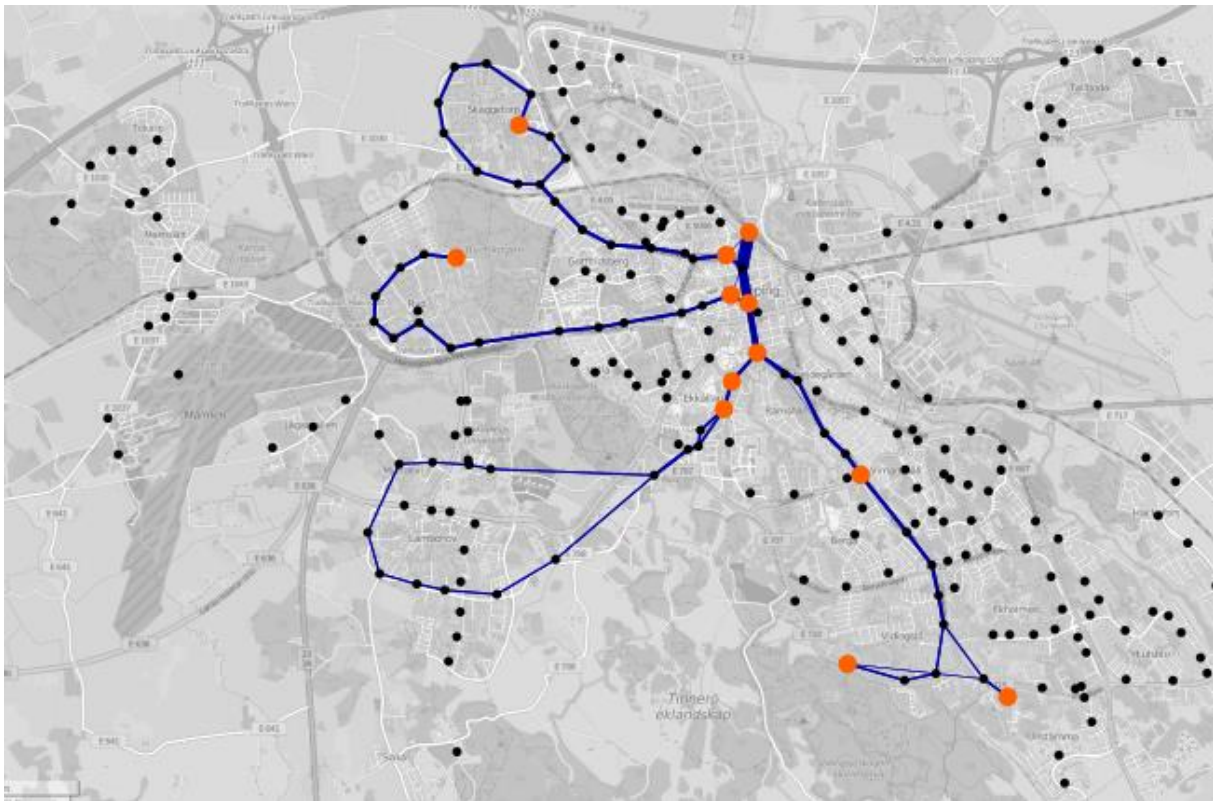
Figure 17 A map of bus line 1, 2, 3 and 4, electrified with only 200 kW charging stations. Red lines show electric roads. Orange dots show charging stations. Black dots show bus stops.
