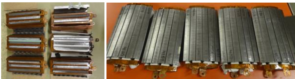
Figure 5.9 Assembled stator segments in prior to heat tests
