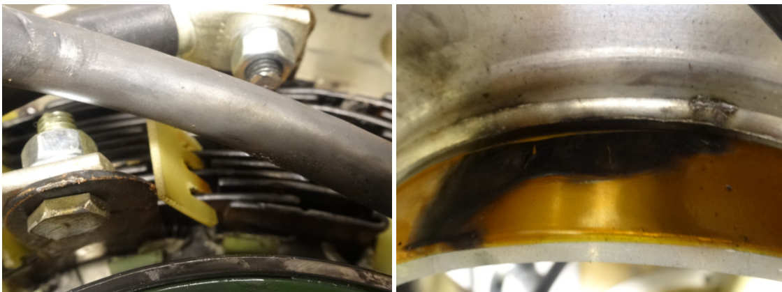
Figure 7.10 Flashover winding (W2) end (NDE or TE)
