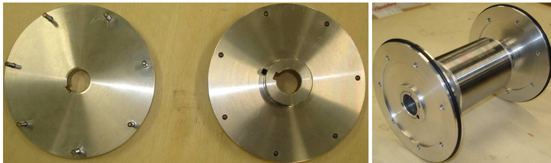
Figure 4.23 Prototyped parts: transmission disks (left) and rotor attached to the inner transmission rings with o-ring.
