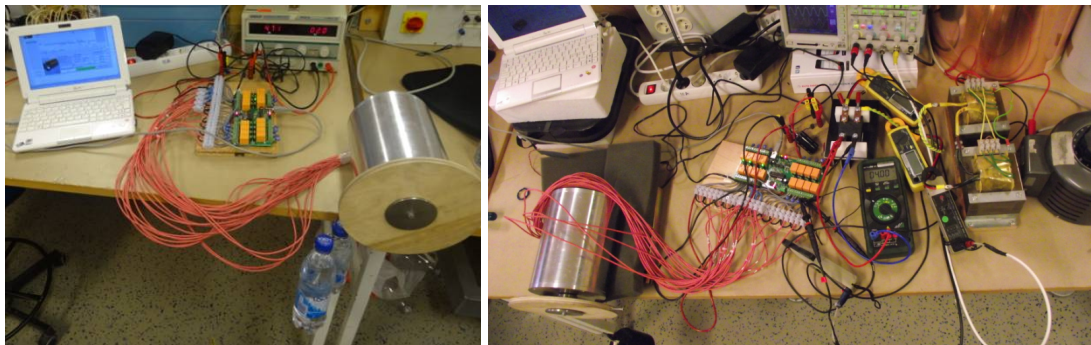
Figure 4.29 Experimental setup on the left figure: from the left 1) PC provides switching sequence to 2) relay card that is 3) supplied from DC voltage source and excites 4) the coils of the prototype motor which is 5) loaded with external weight on the load wheel. Rectified ac supply is used on the right figure.
