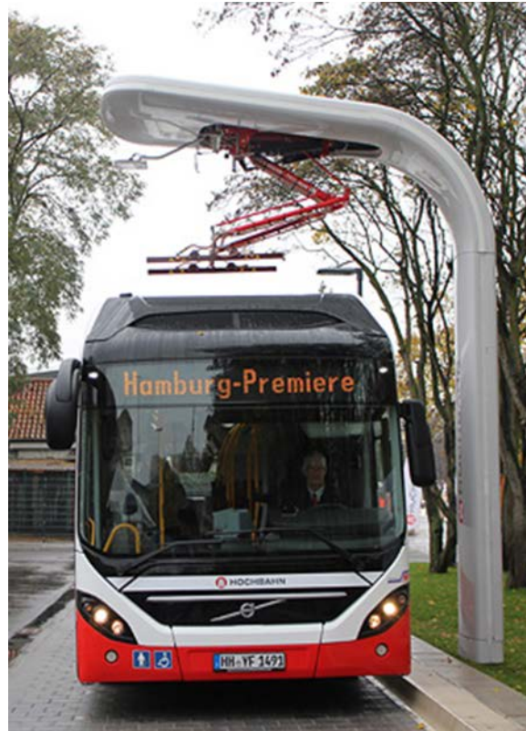
Figure 1 An example of a charging system from Siemens. http://www.siemens.com/press/IM2014110115MOEN
