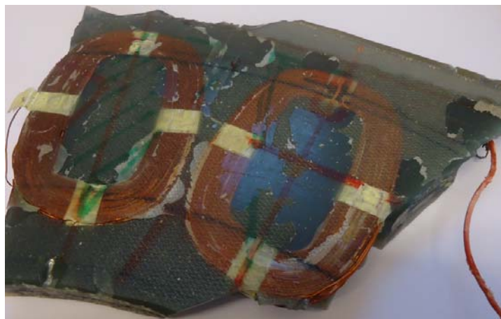
Figure 3.3 Two-coils from the 18-coil 24-pole machine
