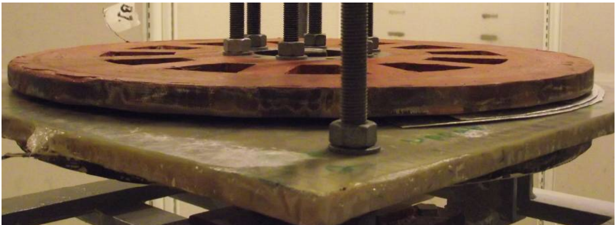
Figure 3.1 Double sided axial flux surface mounted permanent magnet synchronous machine (AFSPMSM)
