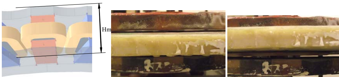
Figure 3.26 Determination of air-gap and montage of the machine with focus on upper and lower air-gap
