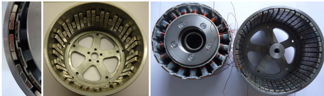
Figure 3.4 Air-gap between rotor and the stator, mounting process of permanent magnets and machine parts in prior to measurements
