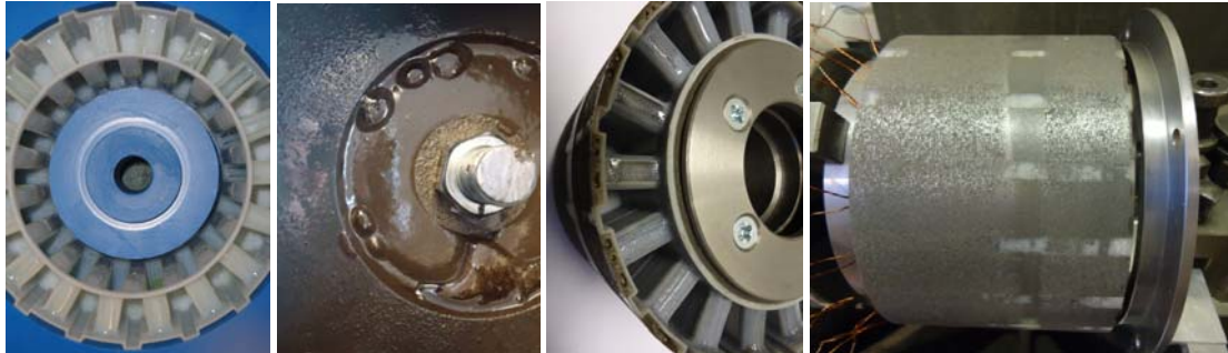
Figure 3.3 The mould with the main insulation system (left), the exchange process (left from the middle) and the ready stator from top and side view
