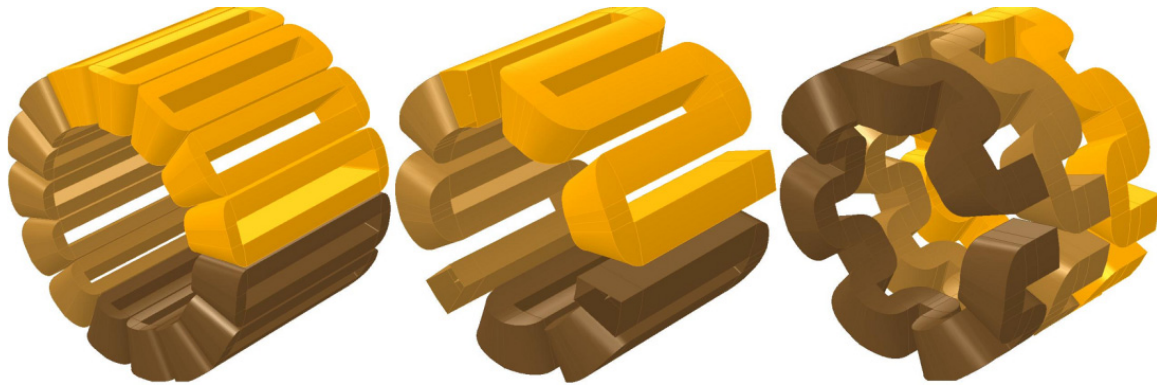
Figure 1.1 Three-phase windings: distributed concentrated (left), circumferentially distributed wave (middle) and axially distributed wave winding (right).
