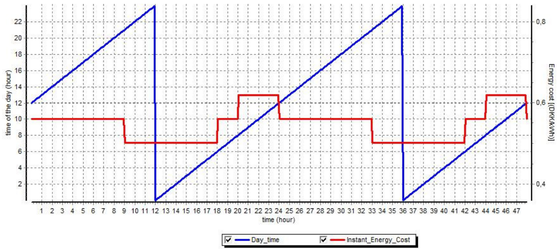
Figure 11: Energy cost and time of day as function of simulation time
