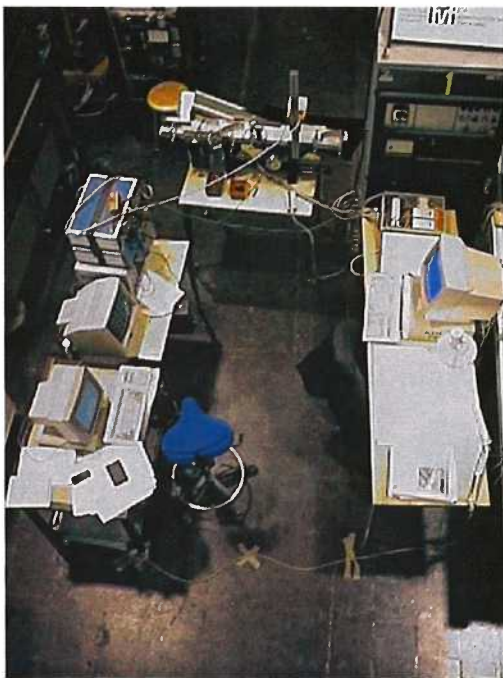
Figure 5 and 6 To the left an overview of the equipment is shown. To the right an object is passing the ultrasonic sensor. (The box contains five sensor elements but in the measurements described only one transmitting and one receiving element was used.) At the conveyer belt to the left of the ultrasonic unit the outlet for pressurized air can be found.
