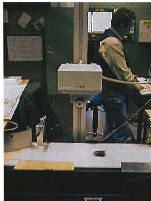
Figure 5 and 6 To the left an overview of the equipment is shown. To the right an object is passing the ultrasonic sensor. (The box contains five sensor elements but in the measurements described only one transmitting and one receiving element was used.) At the conveyer belt to the left of the ultrasonic unit the outlet for pressurized air can be found.
