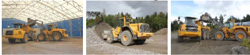
Figure 5 , the three different applications measured. From the right; short loading cycle gravel, load and carry gravel and short loading cycle rock.
