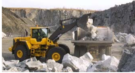
Figure 1, a production machine wheel loader in a bucket application, loading blasted shot rock from face.
