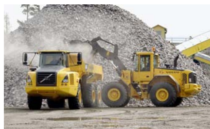
Figure 2, a wheel loader loading an articulated hauler.
