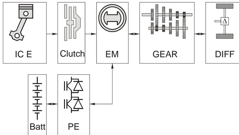
**Figure 6, a schematic picture of parallel hybrid [19].**
