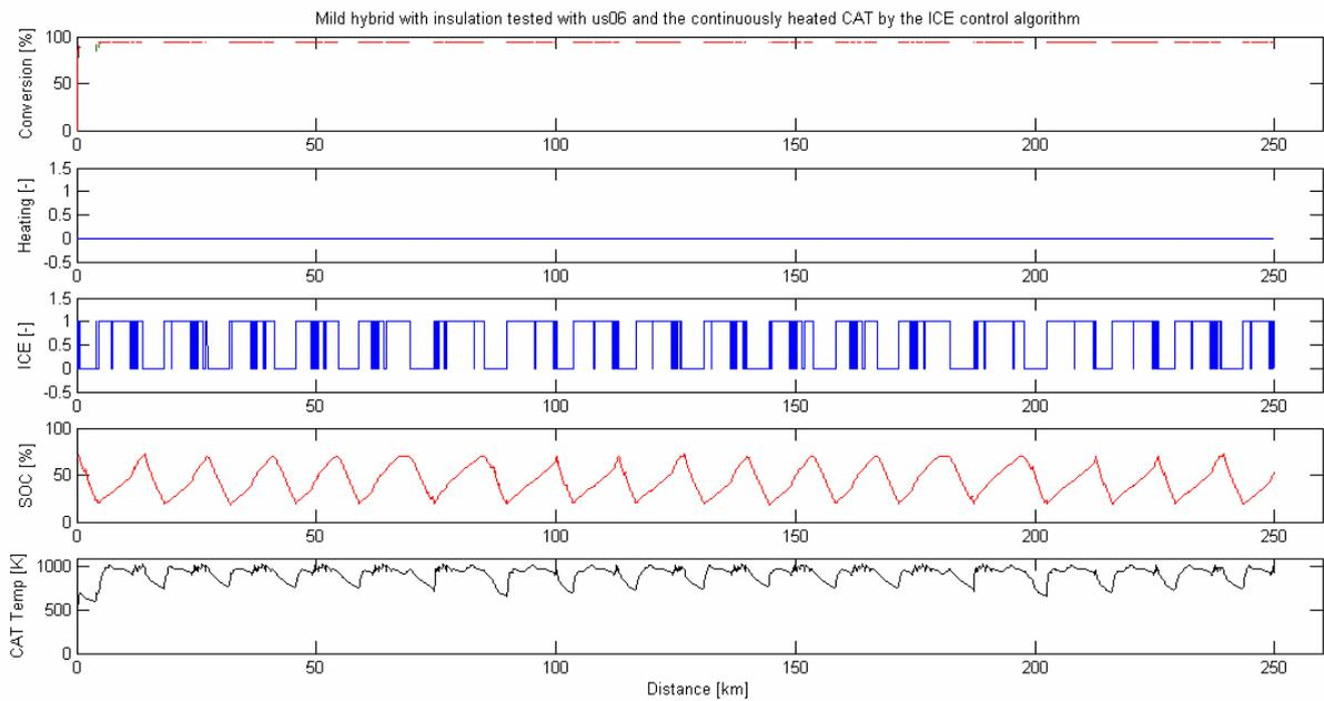
**Figure 20, simulation of a mild hybrid with insulation tested with us06 and the continuously heated catalyst by the internal combustion engine control algorithm.**
