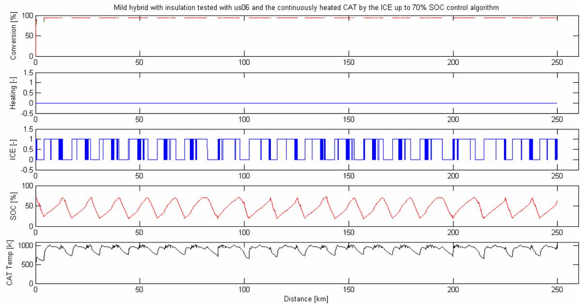
**Figure 22, simulation of a mild hybrid with insulation tested with us06 and the continuously heated catalyst by the internal combustion engine up to 70% state of charge control algorithm.**
