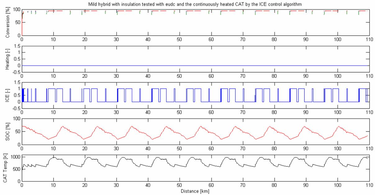
**Figure 19, simulation of a mild hybrid with insulation tested with eudc and the continuously heated catalyst by the internal combustion engine control algorithm.**
