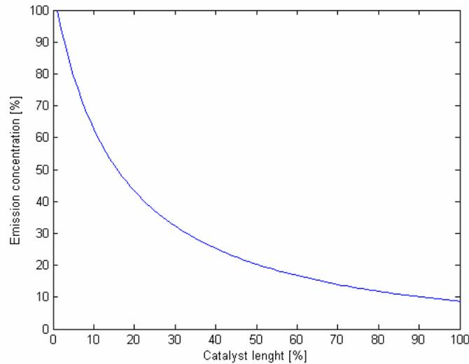
**Figure 4, the emission concentration in the catalyst.**
