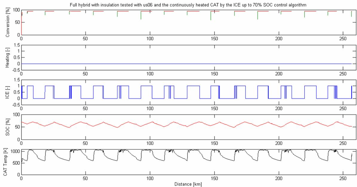
**Figure 32, simulation of a full hybrid with insulation tested with us06 and the continuously heated catalyst by the internal combustion engine up to 70% state of charge control algorithm.**
