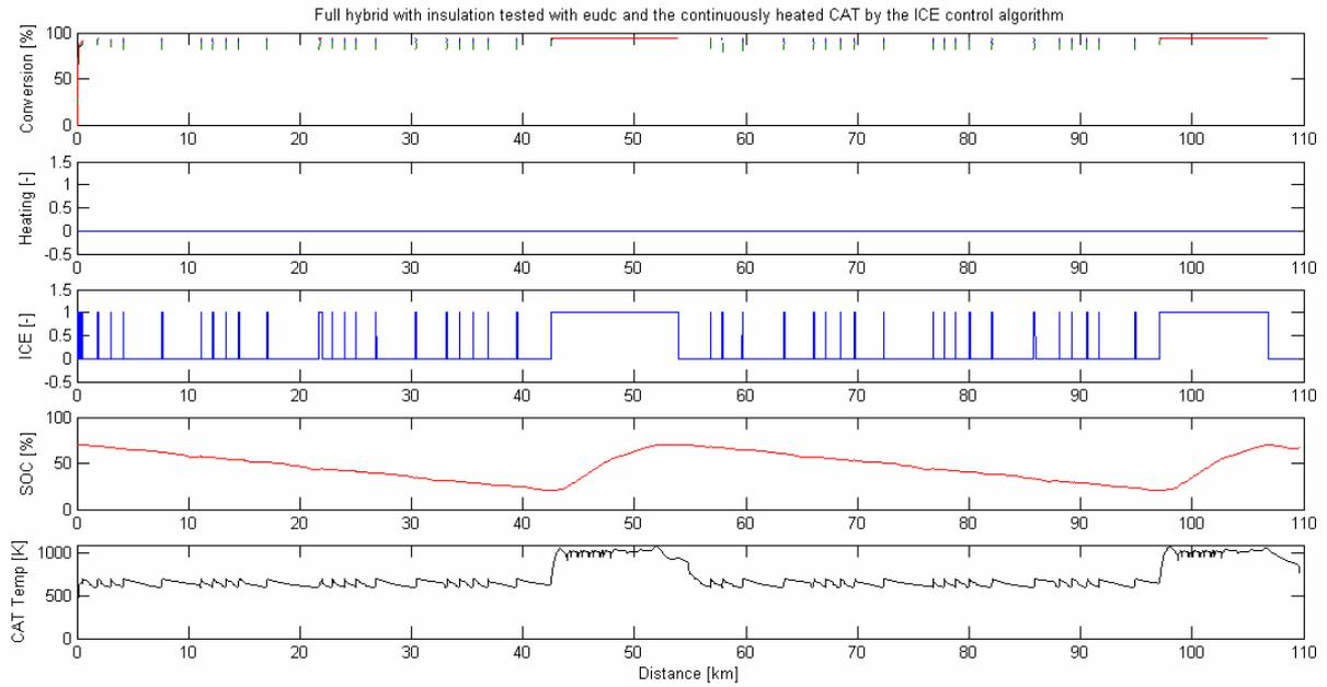
**Figure 29, simulation of a full hybrid with insulation tested with eudc and the continuously heated catalyst by the internal combustion engine control algorithm.**
