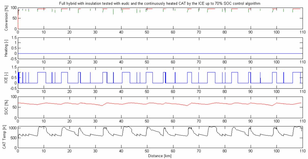
**Figure 31, simulation of a full hybrid with insulation tested with eudc and the continuously heated catalyst by the internal combustion engine up to 70% state of charge control algorithm.**
