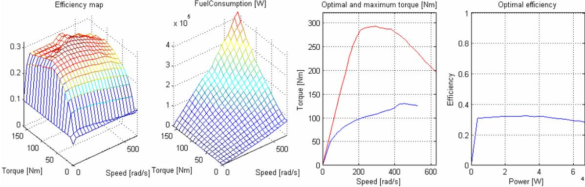
**Figure 10, internal combustion engine properties.**
