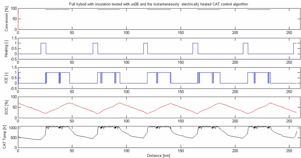
**Figure 28, simulation of a full hybrid with insulation tested with us06 and the instantaneously electrically heated catalyst control algorithm.**
