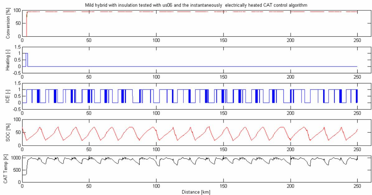
**Figure 18, simulation of a mild hybrid with insulation tested with us06 and the instantaneously electrically heated catalyst control algorithm.**
