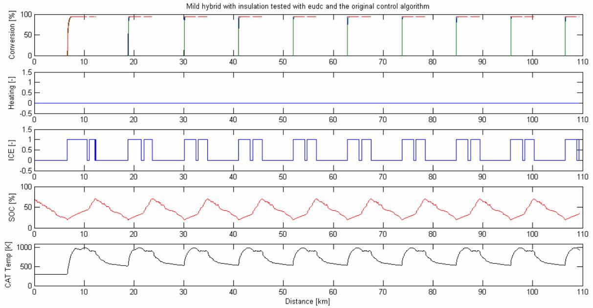
**Figure 13, simulation of a mild hybrid with insulation tested with eudc and the original control algorithm.**
