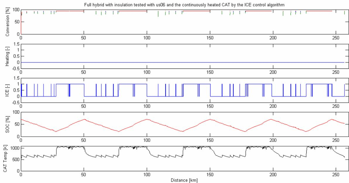
**Figure 30, simulation of a full hybrid with insulation tested with us06 and the continuously heated catalyst by the internal combustion engine control algorithm.**
