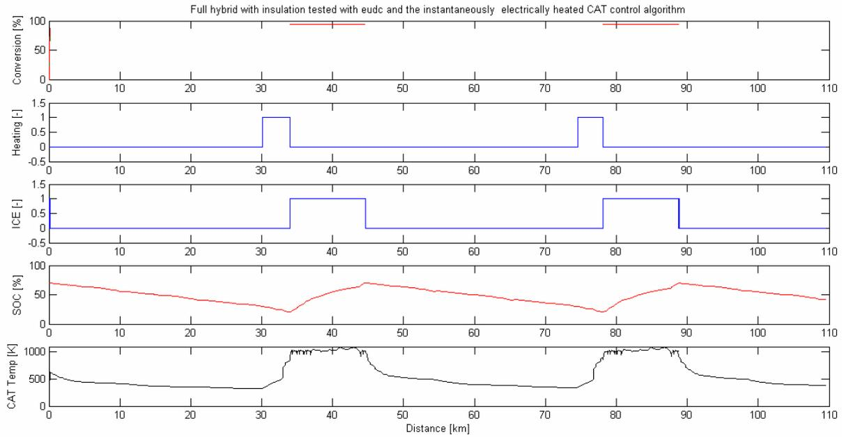
**Figure 27, simulation of a full hybrid with insulation tested with eudc and the instantaneously electrically heated catalyst control algorithm.**
