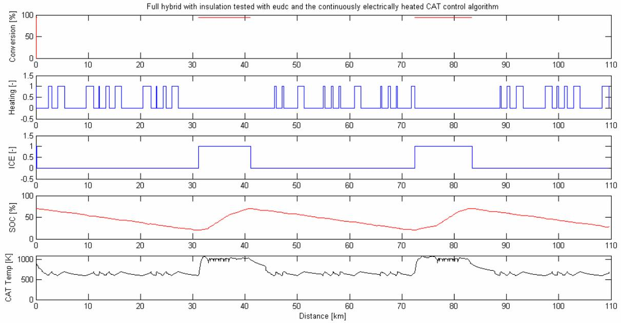
**Figure 25, simulation of a full hybrid with insulation tested with eudc and the continuously electrically heated catalyst control algorithm.**
