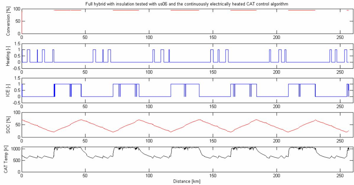
**Figure 26, simulation of a full hybrid with insulation tested with us06 and the continuously electrically heated catalyst control algorithm.**
