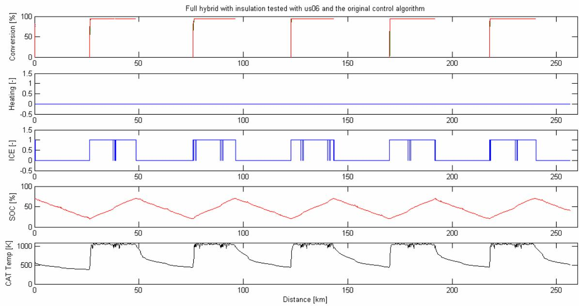
**Figure 24, simulation of a full hybrid with insulation tested with us06 and the original control algorithm.**
