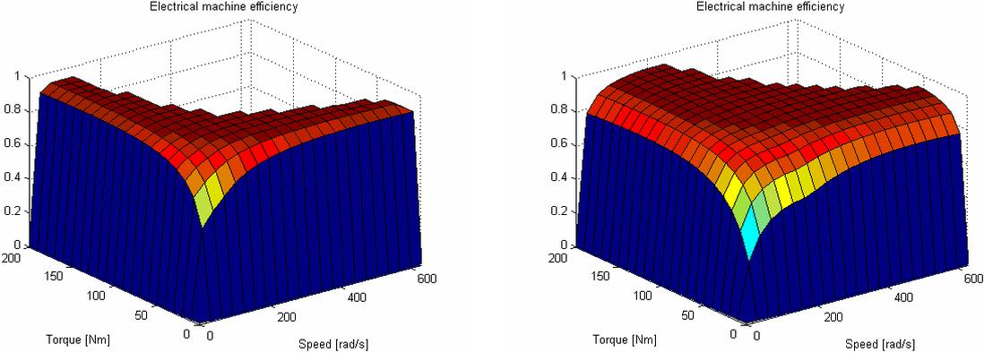
**Figure 11, electrical machines properties.**
