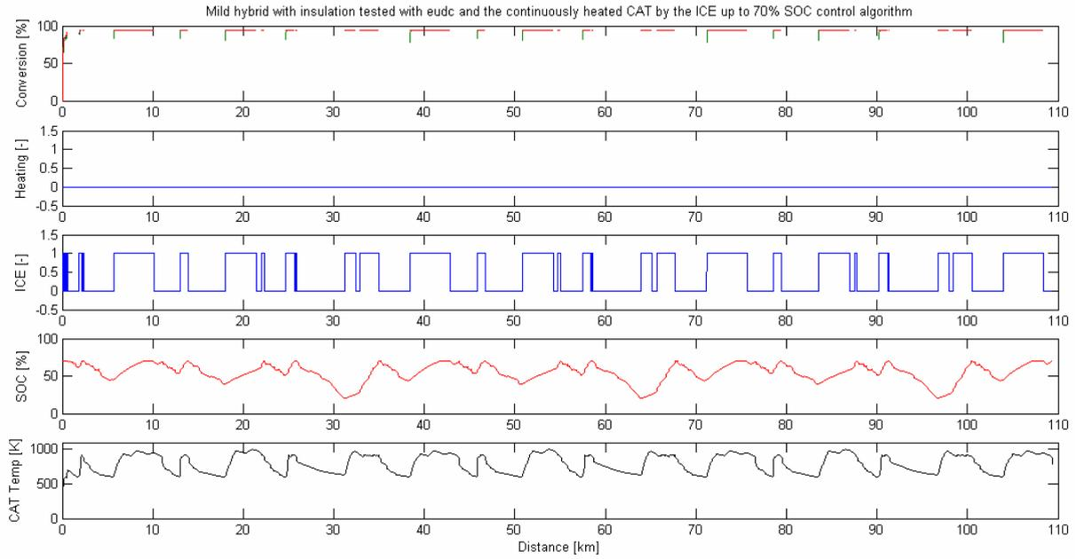
**Figure 21, simulation of a mild hybrid with insulation tested with eudc and the continuously heated catalyst by the internal combustion engine up to 70% state of charge control algorithm.**
