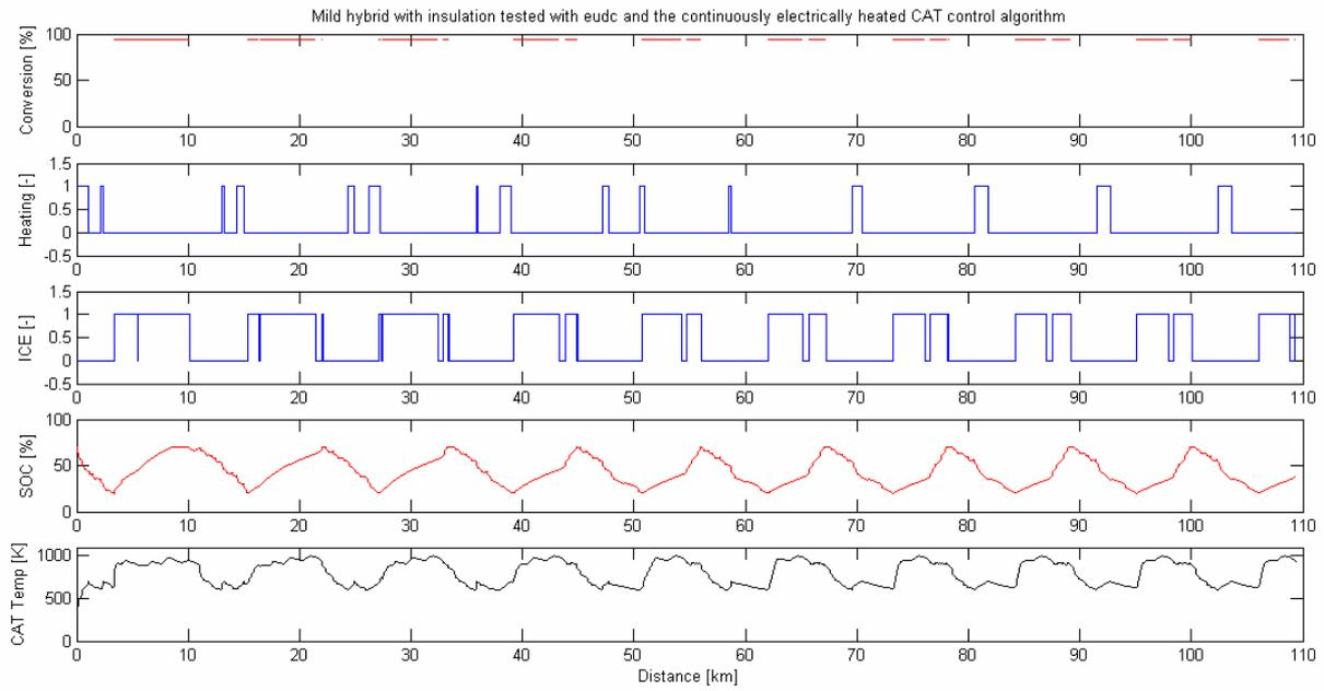
**Figure 15, simulation of a mild hybrid with insulation tested with eudc and the continuously electrically heated catalyst control algorithm.**
