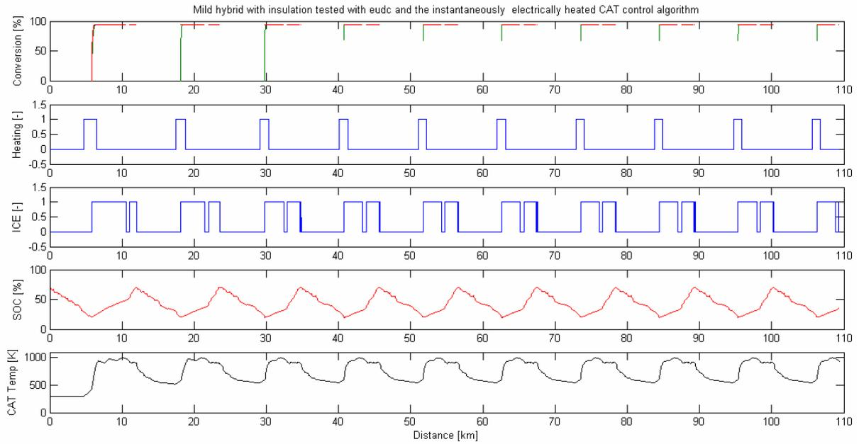
**Figure 17, simulation of a mild hybrid with insulation tested with eudc and the instantaneously electrically heated catalyst control algorithm.**
