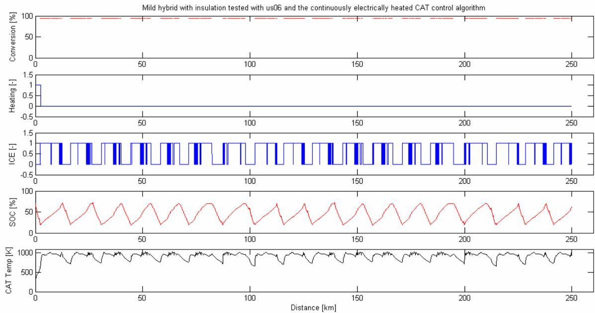
**Figure 16, simulation of a mild hybrid with insulation tested with us06 and the continuously electrically heated catalyst control algorithm.**
