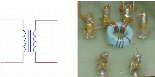
Figure 16.2. Schematic and a real life component view of a signal transformer.
