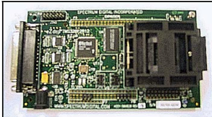
**Figure 2.1-1: Picture of the development card (black case to the right holds the DSP)**
