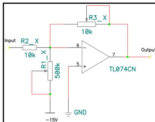
Figure 3.3-3: Used configuration for a *TL074*
