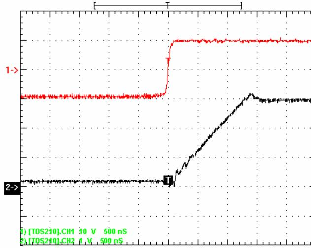
Figure A.10-1: Total delay in an ADC Circuit (Rise time)
