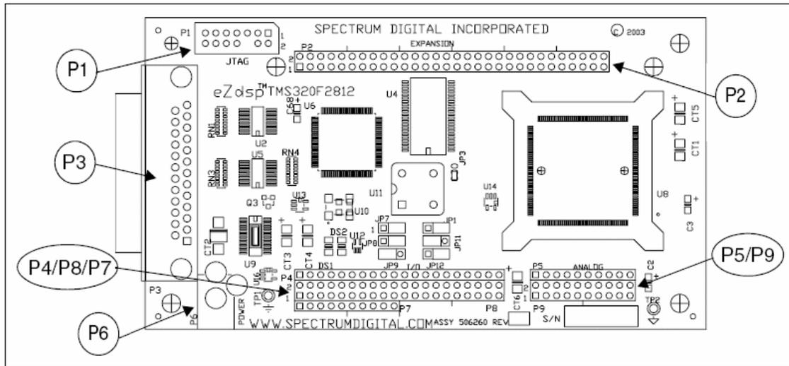
Figure E.3-1: PCB layout of the DSP development board [9.41]
