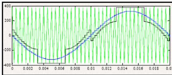
**Figure 5.4-4: Reduced Switching Modulation [9.46]**
