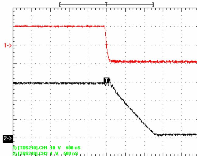
Figure A.10-2: Total delay in an ADC Circuit (Fall time)
