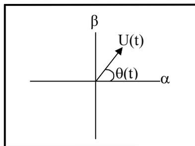
**Figure 5.2-3: Three-phase representations in a  $[\alpha, \beta]$ -frame**
