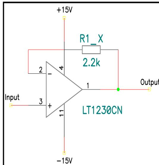
Figure 3.3-5: Used configuration for a LT1230
