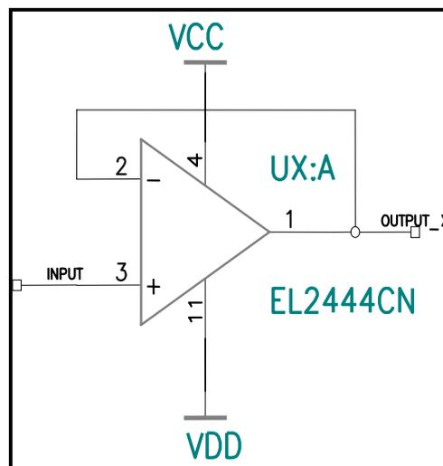
Figure 3.3-4: Used configuration for an EL2444<sup>1</sup>
