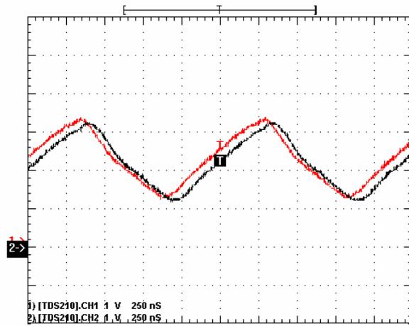
Figure A.8-2: An EL2044 vs. a LM347 at 0.9 MHz
