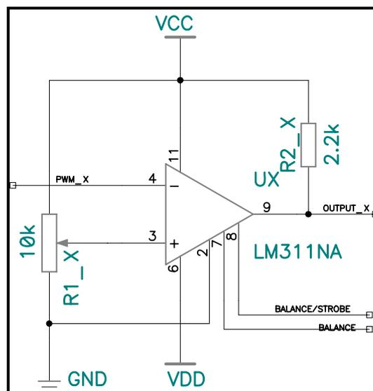
Figure 3.3-1: Used configuration for a LM311
