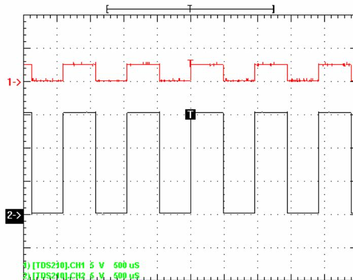
Figure A.2-2: A LM311 with pull-up
