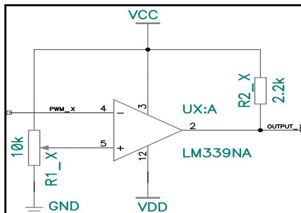
Figure 3.3-2: Used configuration for a LM339
