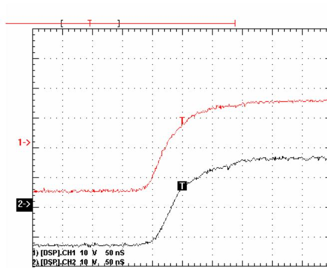
**Figure A.9-1: Internal delay of LT1230CN**
