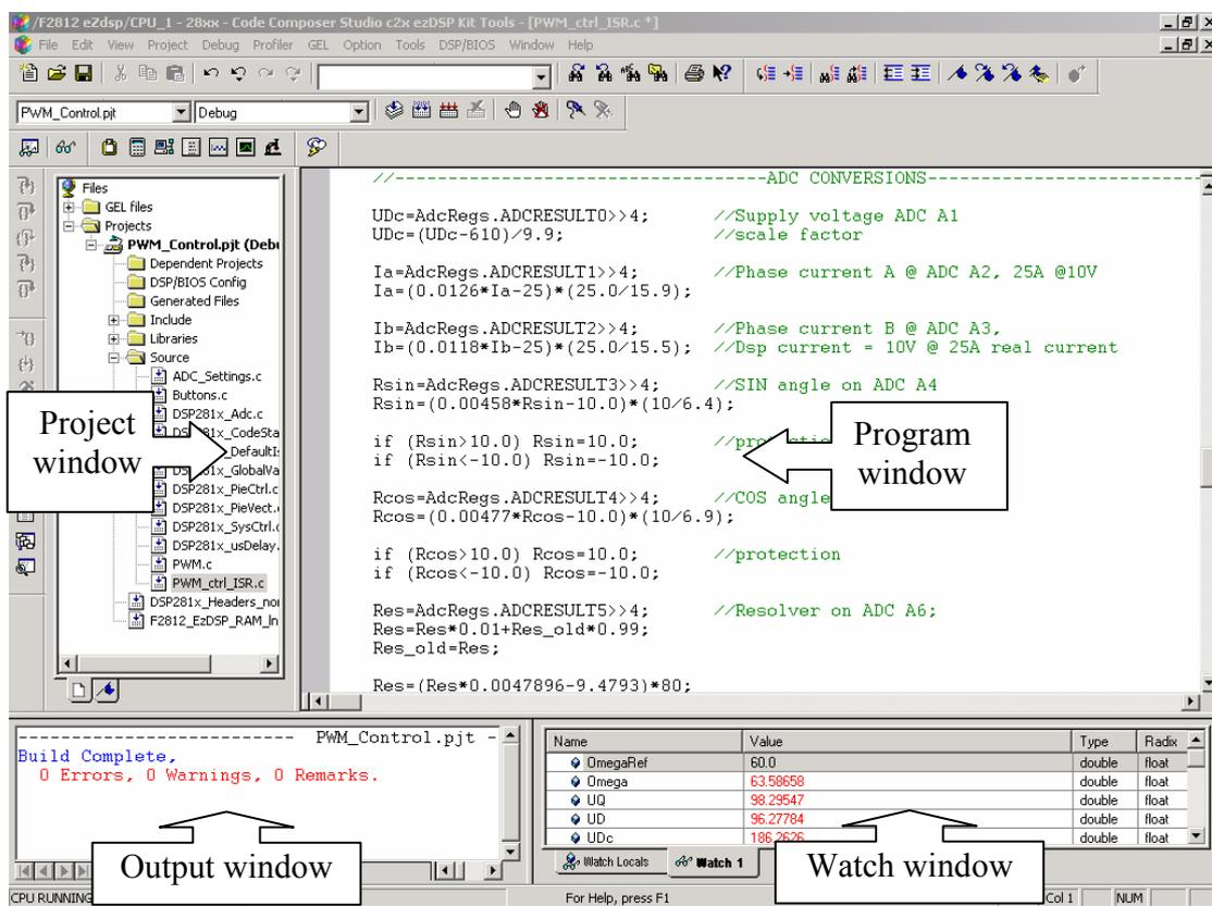
Figure 2.2-1 Snapshot of CCS programming interface
