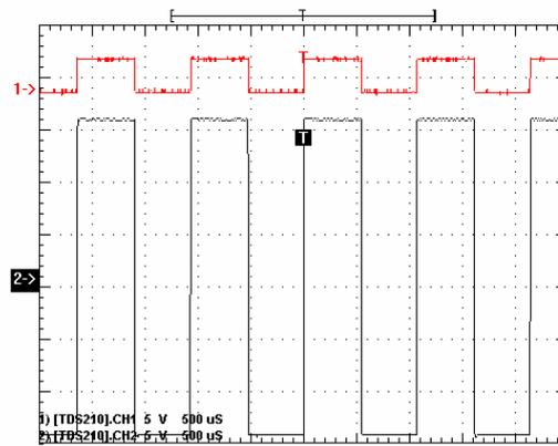
Figure A.4-2: A LM339 with pull-up
