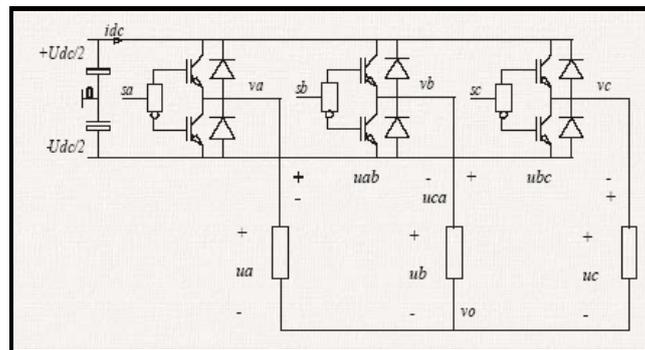
Figure 5.2-1: Three-phase converter [9.42]
