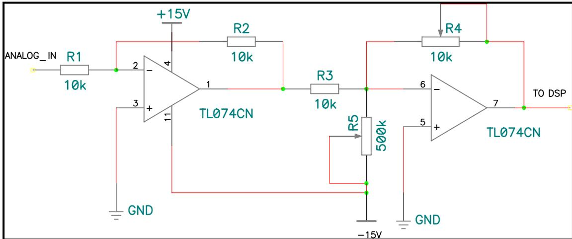
**Figure 3.4-1: ADC circuit**
