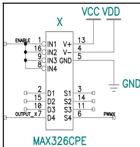
Figure 3.3-6: Used configuration for a MAX 326
