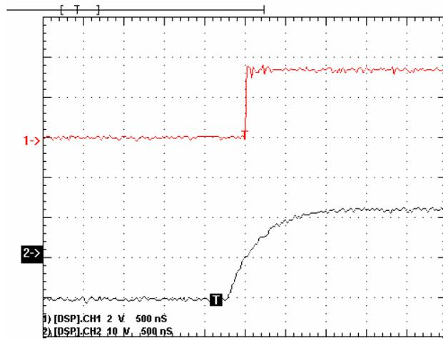
Figure A.10-4: The total delay in a PWM channel (Fall time)
