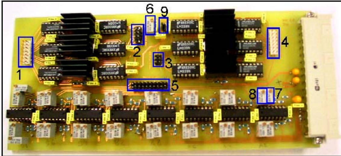
Figure E.3-2: Important spots on the interface card
