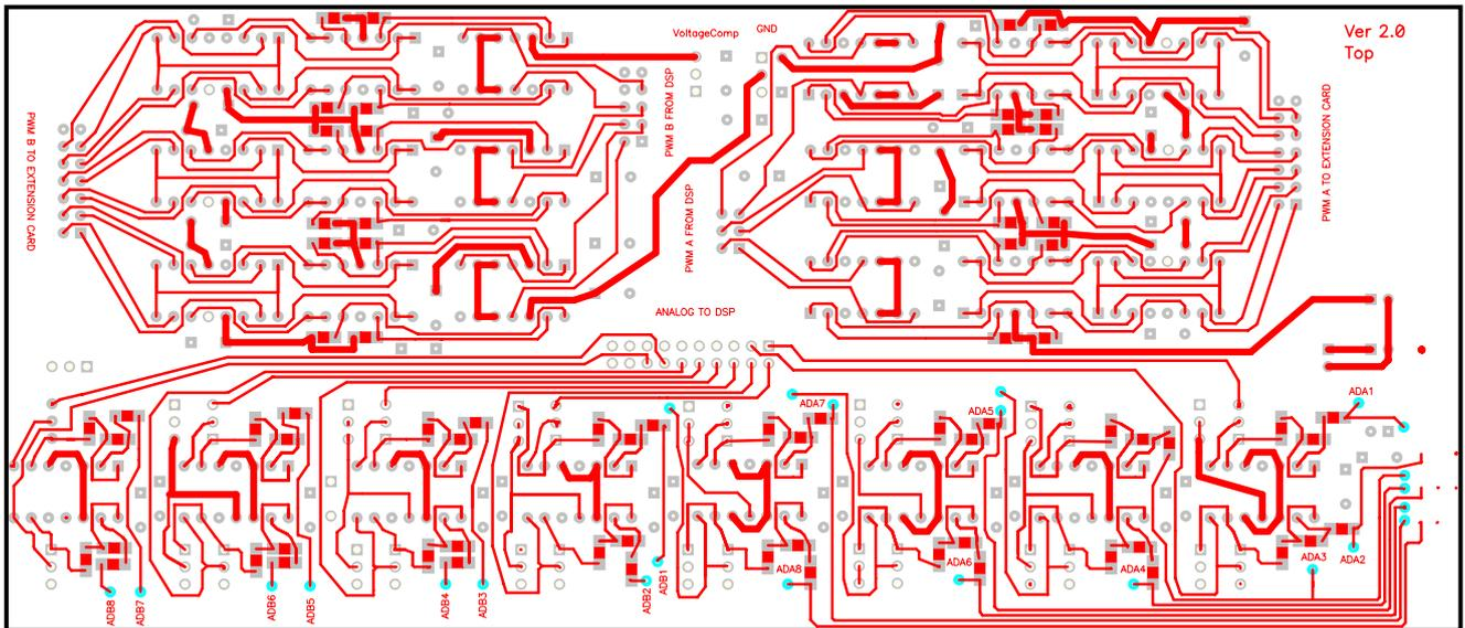
Figure D.2-1: Power Electronic Card, Top layer
