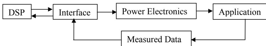
**Figure 1.1-2: Controller outline for the DSP system**
