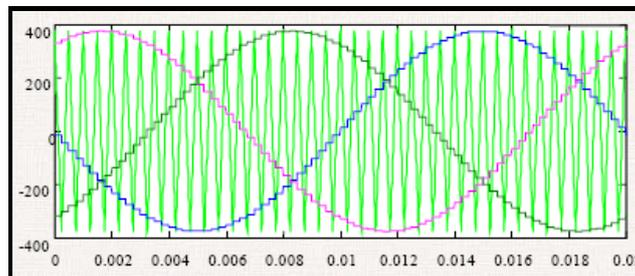
Figure 5.4-2: Sinusoidal Modulation [9.44]
