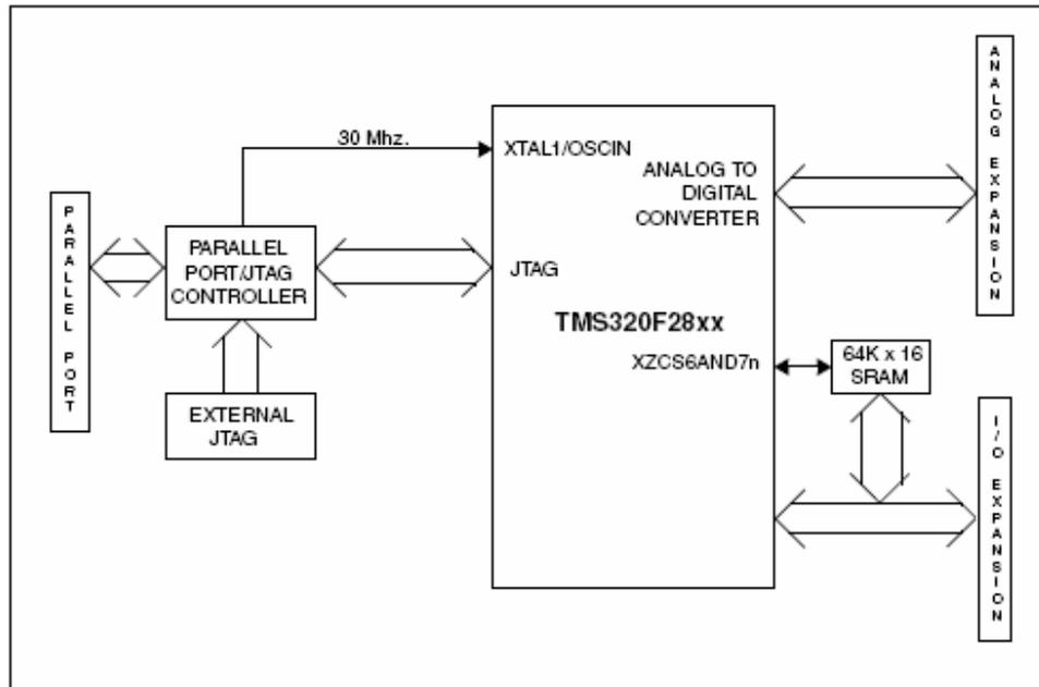
Figure 2.2-2: Block diagram of the development card [9.41]
