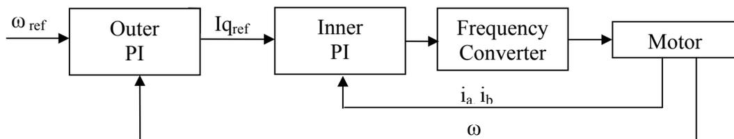
Figure 7.2-1: PMSM Controller layout
