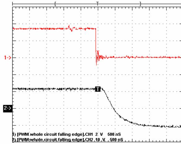
Figure A.10-3: The total delay in a PWM channel (Fall time)
