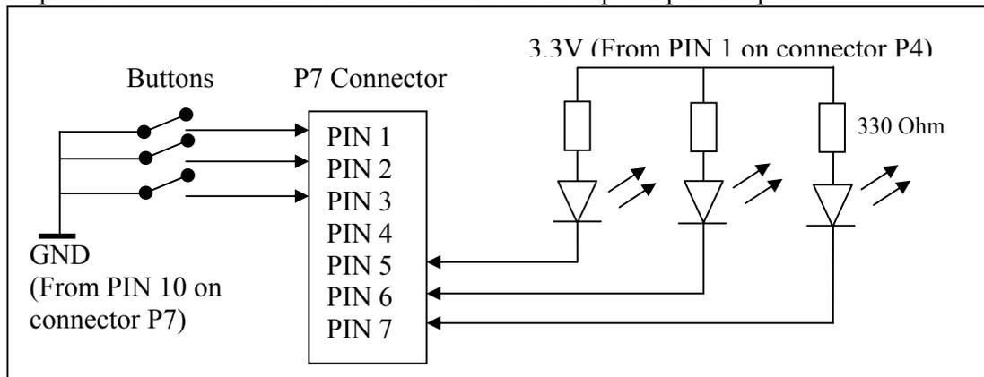
**Figure E.1-2: Schematics of LEDs and Button connections**
