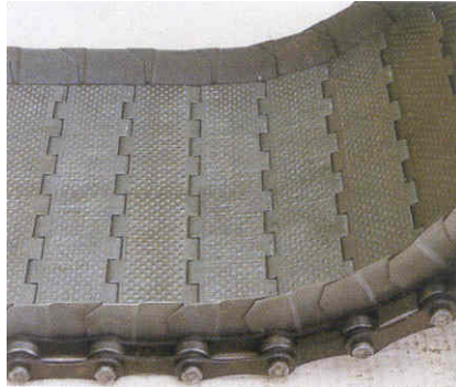
Figure 12: Hinged steel belt to conveyors.
