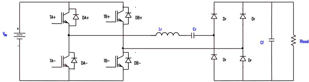
Figure 2.6 A series resonant DC-DC full bridge converter.
