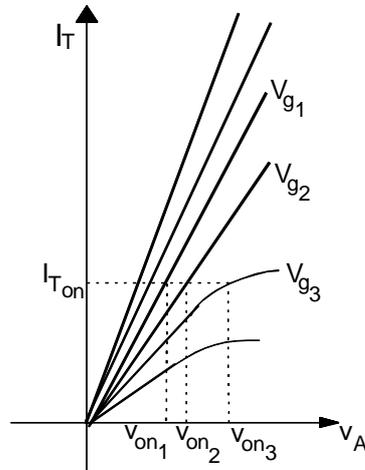
**Figure 5.5** On-state voltage at a given collector current for different gate voltages.
