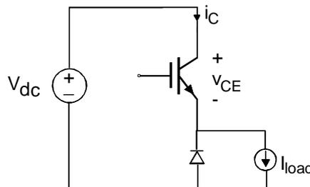
Figure 2.1 The step down converter.
