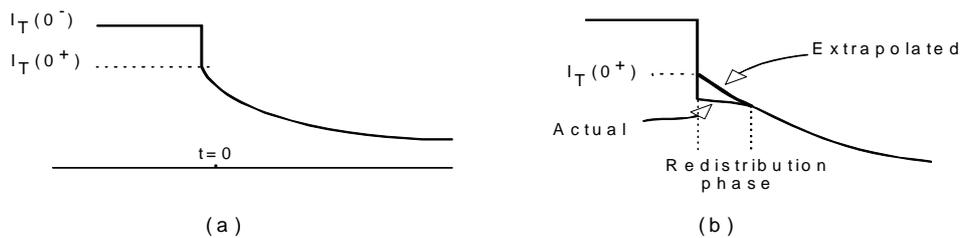
Figure 5.3 Constant anode voltage turn-off with a) current waveform indicating current levels before and after the rapid fall of the MOSFET current, and b) the redistribution phase and the extrapolation of  $I_T(0^+)$ .
