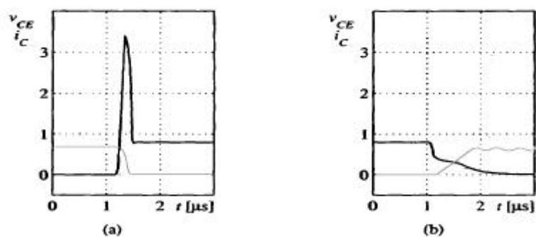
**Figure 2.4** Normalised transistor current (black) and voltage (grey) during a) turn-on and b) turn-off of the power transistor in the step down converter with a capacitive snubber. Note the collector current peak at turn-on, and the simultaneously change of the collector current and collector-emitter voltage at turn-off [21].
