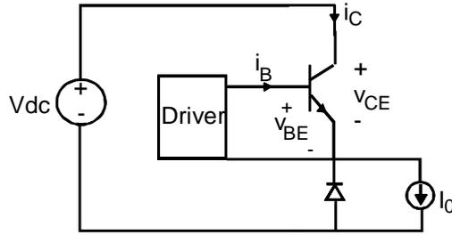
Figure 3.9 Inductively loaded BJT switching circuit with a diode clamp.
