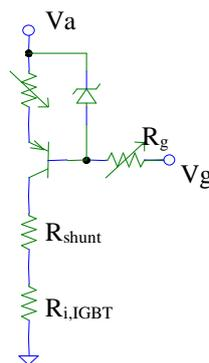
Figure 5.10 Schematic circuit configuration of the current generator.
