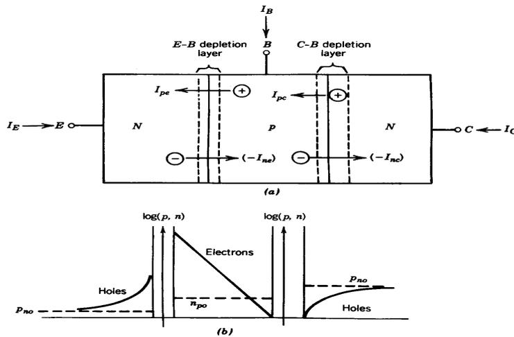
Figure 3.7 a) Carrier transport in a simplified model of the BJT and b) stored charge distribution in the normal active region [20].
