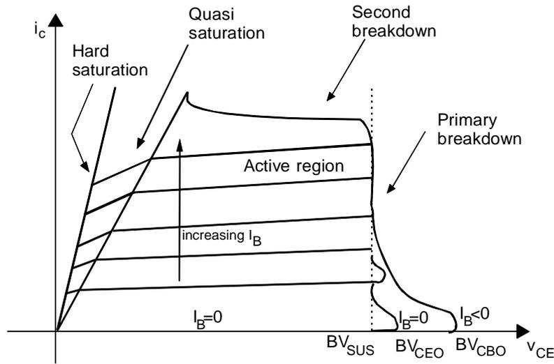
Figure 3.6 The  $i$ - $v$  characteristics of a BJT.
