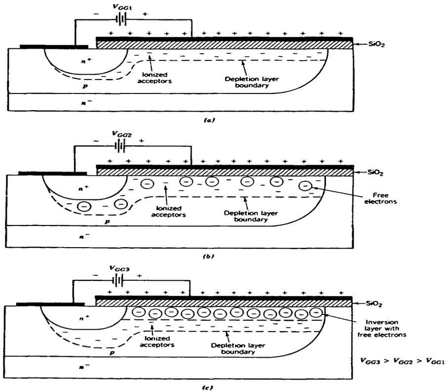
Figure 3.14 Formation of the a) depletion layer and b) c) inversion layer, as the gate-source voltage is increased [20].
