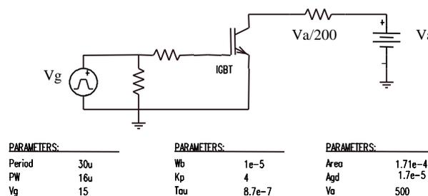
**Figure 6.1** Test circuit for the IGBT parameters.
