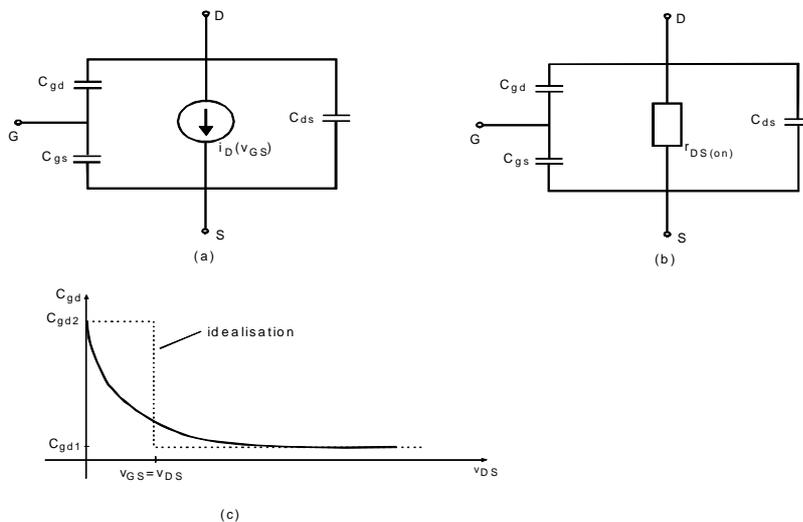
Figure 3.15 Equivalent circuits of MOSFET for transient analysis a) in cut-off and active region b) in ohmic region and c) the variation of gate-drain capacitance with drain-source voltage.
