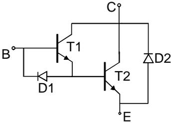
Figure 3.5 Darlington connection where  $\beta = \beta_{T1} \beta_{T2} + \beta_{T1} + \beta_{T2}$ . D1 is added to aid turn-off and D2 for full bridge applications.
