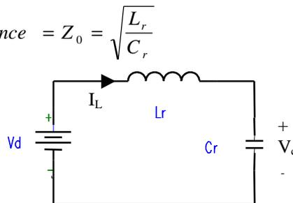
Figure A.1 The undamped series resonant circuit.
