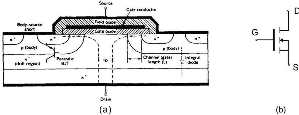
Figure 3.12 a) Vertical structure of  $n$ -channel MOSFET. The thickness of the layers is not according to scale [20] b) circuit symbol.
