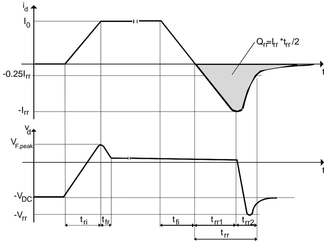
Figure 3.3 Switching trajectories for the power diode.
