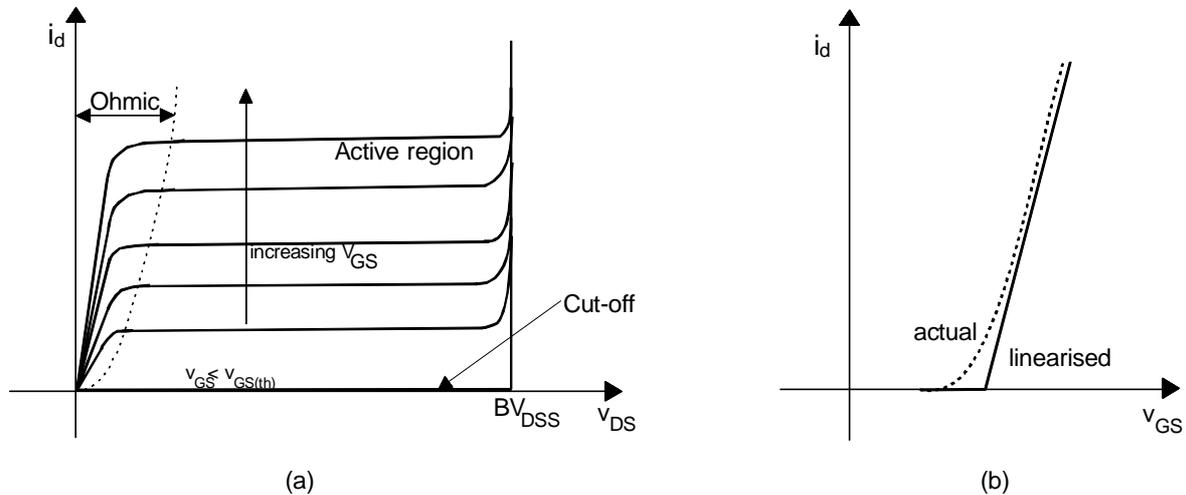
Figure 3.13 a)  $i$ - $v$  characteristics and b) transfer function of the MOSFET.
