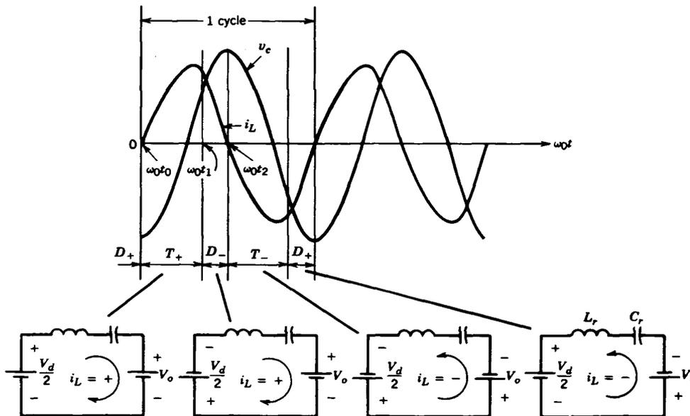
Figure 2.8 Series resonant converter, continuous conduction mode ( $\omega_s > \omega_0$ ) [20].
