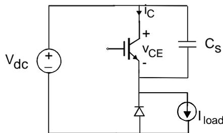
**Figure 2.3** The step down converter with a capacitive snubber.
