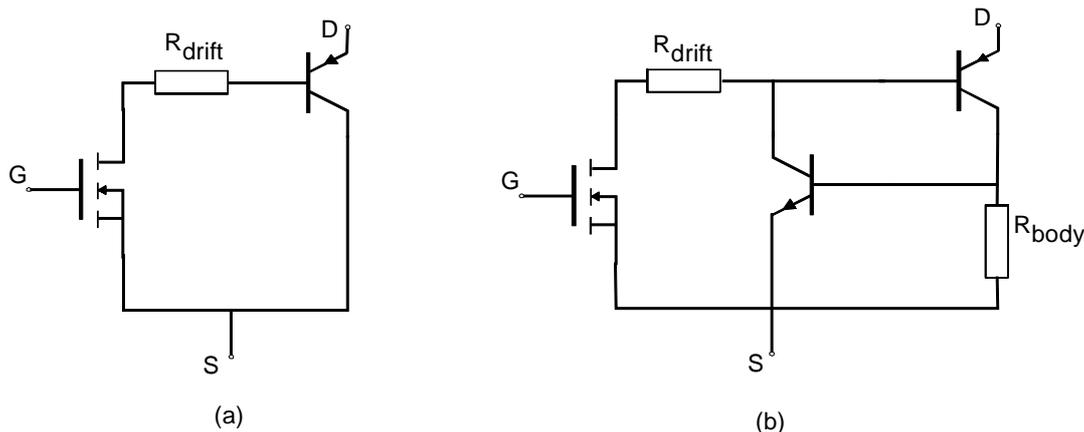
Figure 3.18 a) Darlington circuit of IGBT b) including parasitic thyristor.
