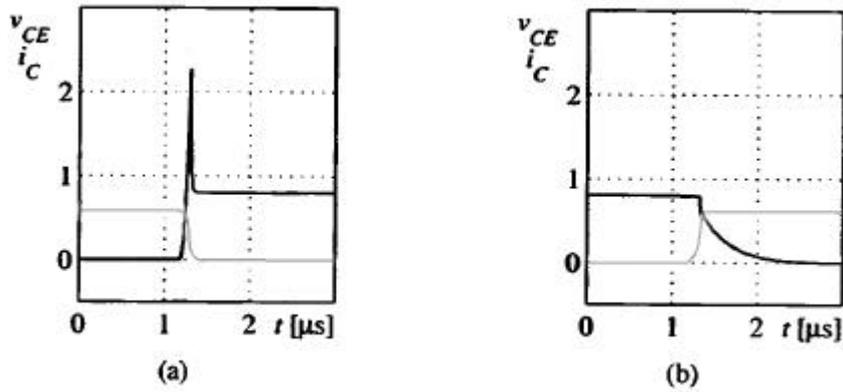
**Figure 2.2** Normalised transistor current (black) and voltage (grey) during a) turn-on and b) turn-off of the power transistor in the step down converter [21].
