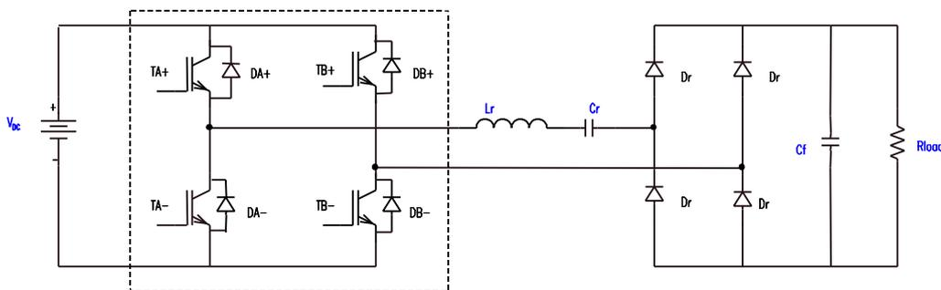
Figure 1.1 The series resonant converter including a full-bridge with IGBTs.
