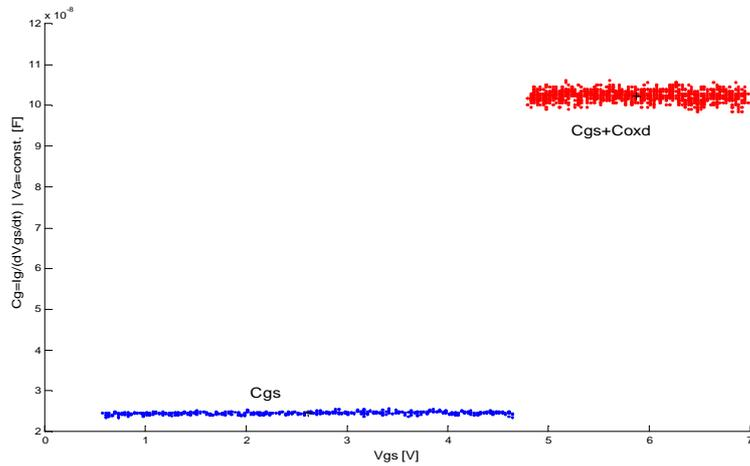
**Figure 5.7** The input capacitance versus gate voltage during the first and third phase of Figure 5.6.
