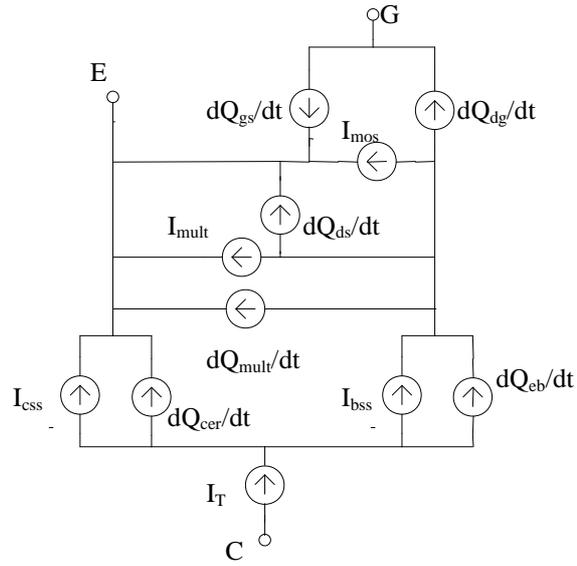
**Figure 4.1** Equivalent circuit of the MicroSim® PSPICE® IGBT model.
