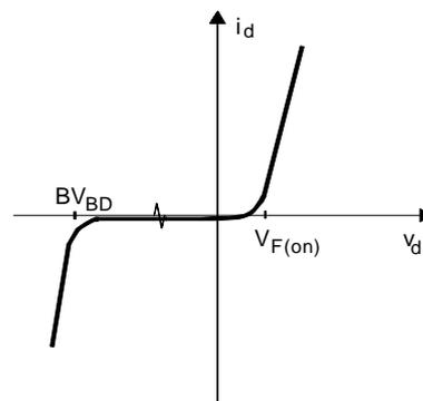
**Figure 3.2** The  $i$ - $v$  characteristic of the power diode.
