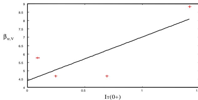
**Figure 5.11** Plot of  $\beta_{tr,v}$  in measurement #2 with a large spread of the data resulting in a poorly fitted least-squares fit.
