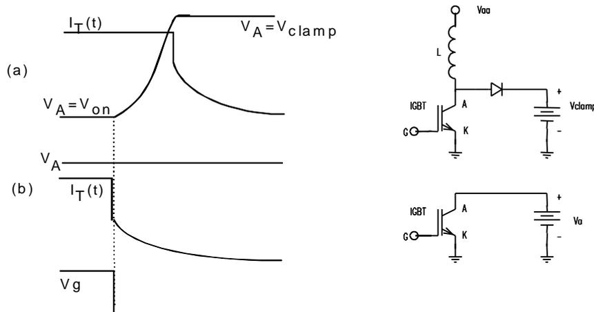
**Figure 5.1** The turn-off switching waveform and circuit configuration for a) The clamped large inductive load circuit b) The constant anode supply voltage.
