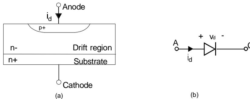
**Figure 3.1** a) Cross section of power diode and b) circuit symbol.
