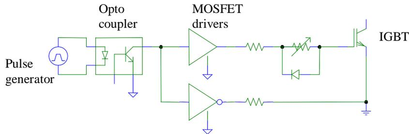
Figure 5.9 Schematic circuit configuration of the gate drive circuit for  $\pm 15$  V supply voltage.
