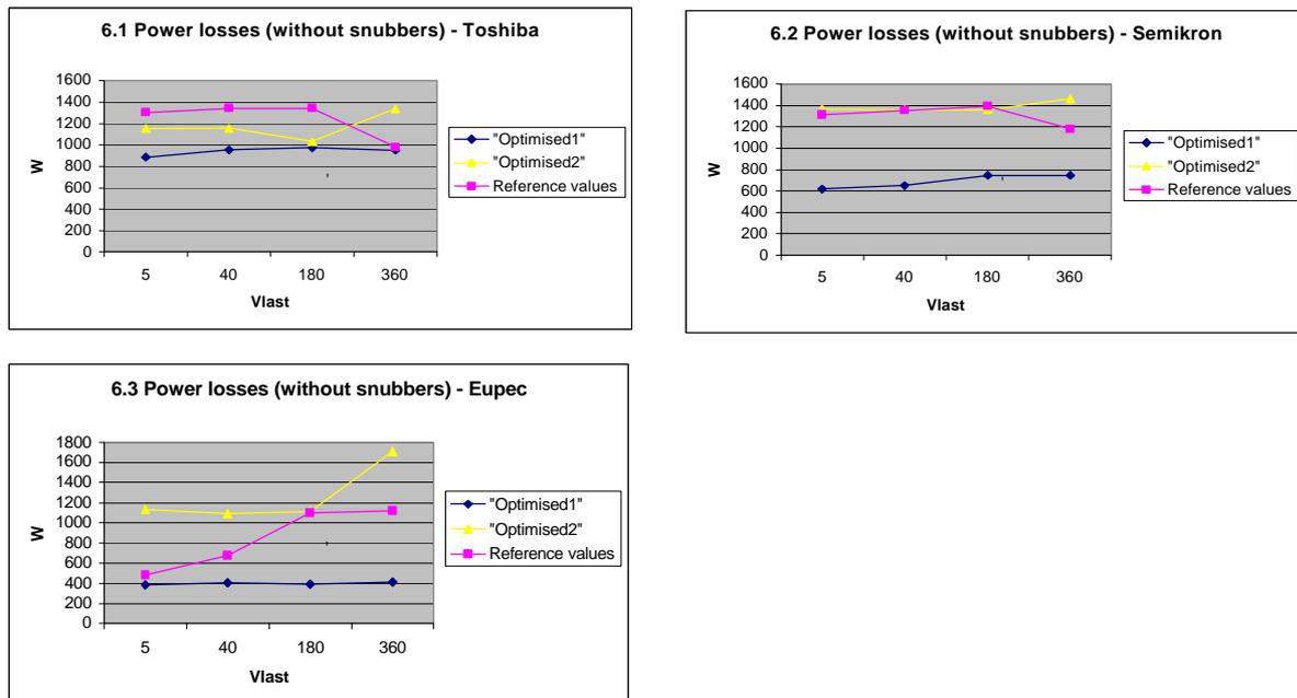
**Diagram 6.1 – 6.3** Power losses with two different parameter sets (“Optimised 1” and “Optimised 2”).
