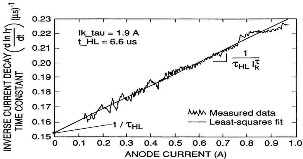
Figure 5.2 Current tail decay rate with  $1/\tau_{HL}$  equal to the extrapolated zero current intercept [7].
