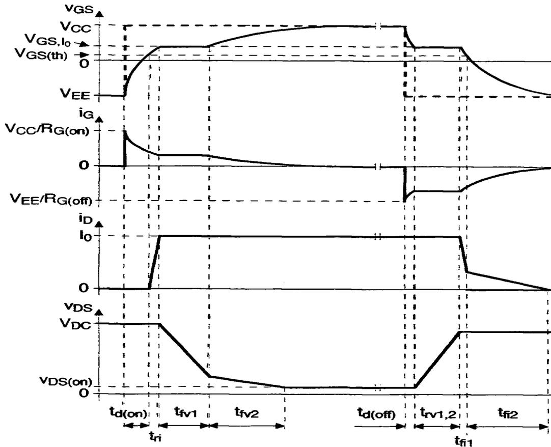
Figure 3.19 Switching transient of the IGBT [22].
