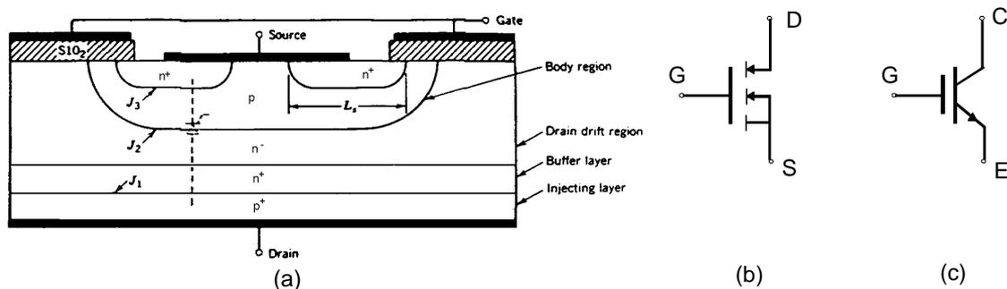
Figure 3.17 a) Vertical cross section of the IGBT [20] and b) c) circuit symbols
