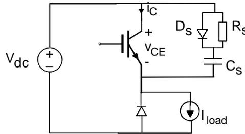
**Figure 2.5** The step down converter with a RCD snubber.
