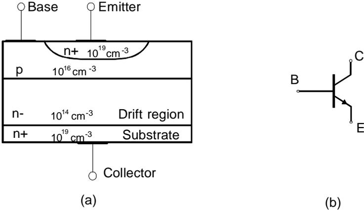
Figure 3.4 a) Vertical structure of *npn* BJT with typical doping densities and b) circuit symbol
