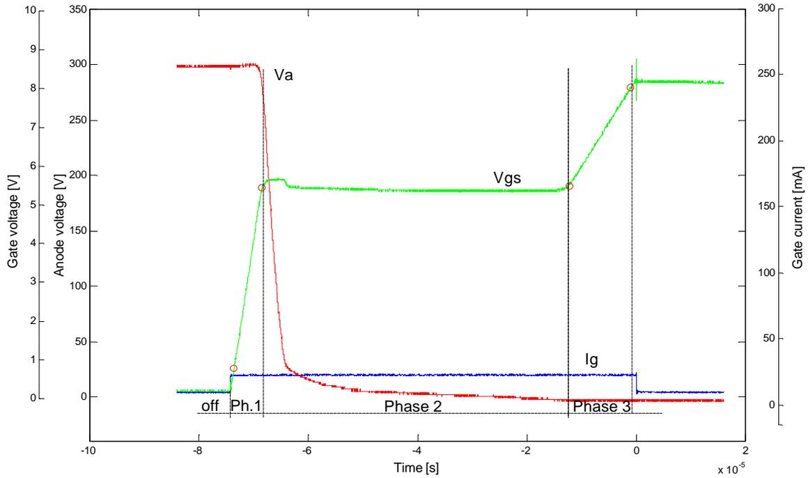
**Figure 5.6** The gate and gate-drain characteristics for a low anode current and nearly constant gate current pulse.
