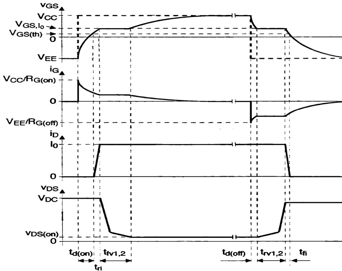
Figure 3.16 Switching transients for the MOSFET [22].
