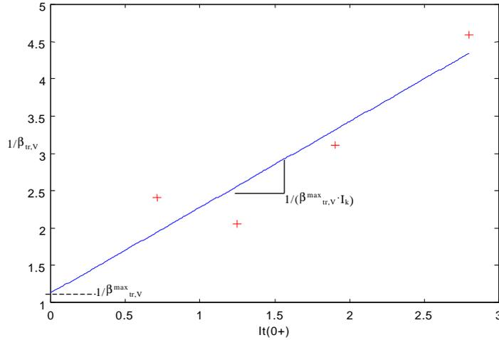
Figure 5.4  $1/\beta_{tr,V}$  versus  $I_T(0^+)$  for 125 V anode voltage, indicating  $\beta_{tr,V}^{\max}$  at zero current intercept.
