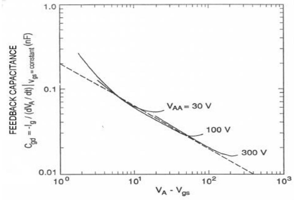
**Figure 5.8** The gate-drain feedback capacitance versus anode-gate voltage for three different supply voltages. The dashed line is fitted to the waveforms of higher voltages due to the approximation in eq. 5.11[7].
