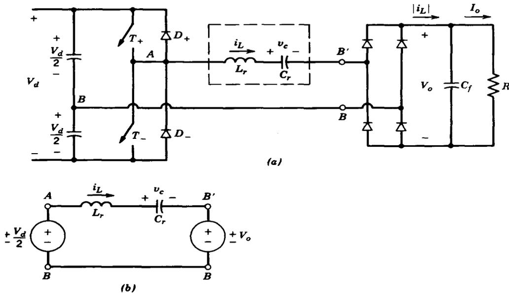
Figure 2.7 Series resonant converter: a) half-bridge b) equivalent circuit[20].
