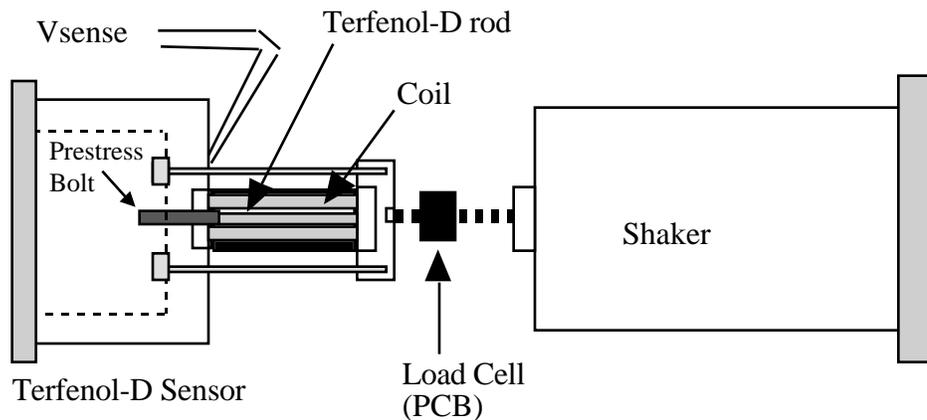
Figure 1: Testing setup for Terfenol-D transducer used as a force sensor.
