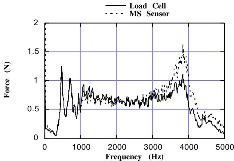
Figure 2: Comparison of the load cell force and force measured by the Terfenol-D sensor using equation 6 versus frequency.
