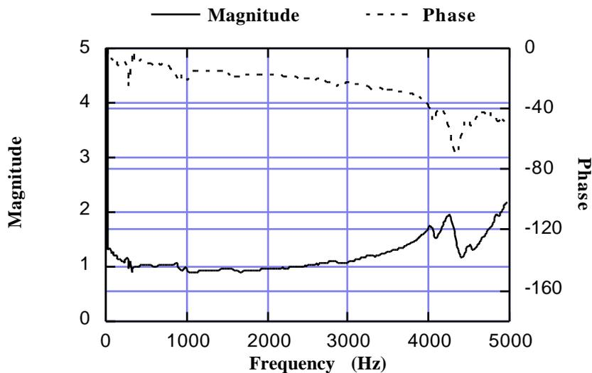
Figure 4: Transfer function between the force measured by the Terfenol-D sensor using equation 6 and the force measured by the load cell.
