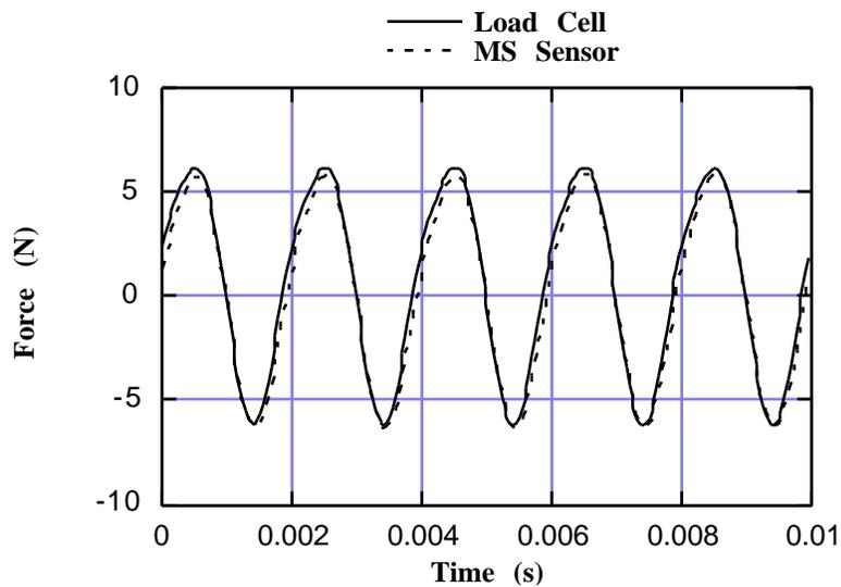
Figure 3: Comparison of time domain force measured by the load cell and measured by the Terfenol-D sensor using equation 6.
