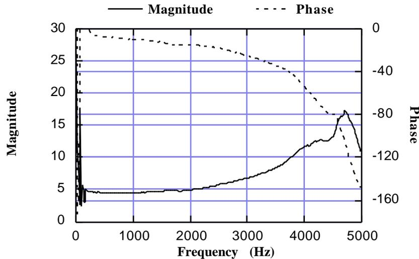
Figure 5: Transfer function between force measured by the Terfenol-D sensor using equation 6 and the force measured by the load cell in blocked free configuration.
