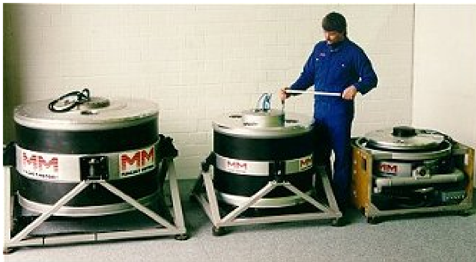
Figure 3.5 Three flywheel energy storages. The peak specifications are 80 MJ / 5 MW for the biggest and 80 MJ / 2.5 MW for the medium sized. The smallest is not known at the time of writing.
