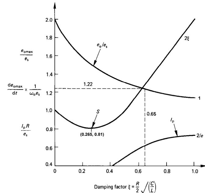
Figure 8.4. Variation of snubber peak voltage,  $e_o$ , maximum  $de_o/dt$ ,  $\dot{S}$ ; and peak current,  $I_p$ ; with L-C-R damping factor  $\xi$ .
