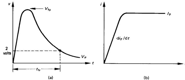
Figure 4.2. Diode forward recovery measurement:
