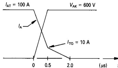
Figure 8.25. Problem 8.1, GTO thyristor tail current characteristics.
