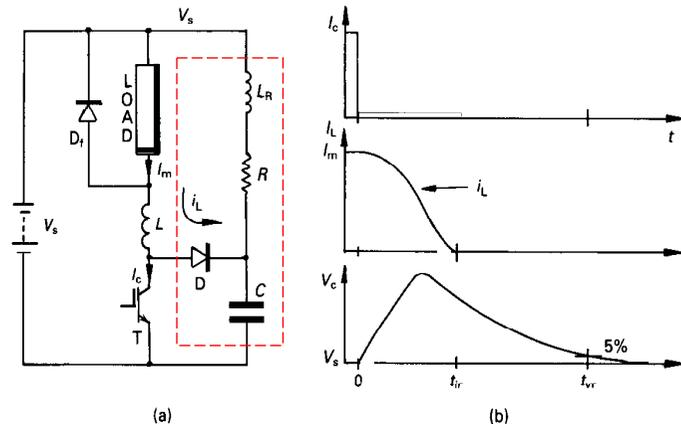
Figure 8.6. Soft voltage polarised clamp:
