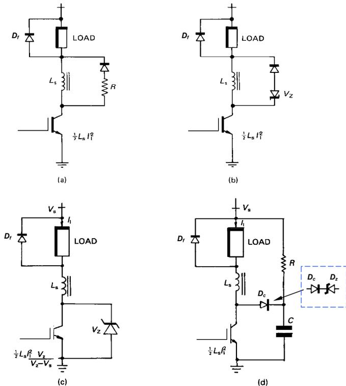
Figure 8.19. Four turn-on snubber modifications for increasing the rate of release of inductor  $L_s$  stored energy: (a) using a power resistor; (b) using a power Zener diode; (c) parallel switch Zener diode,  $V_z > V_s$ ; and (d) using a soft voltage clamp.
