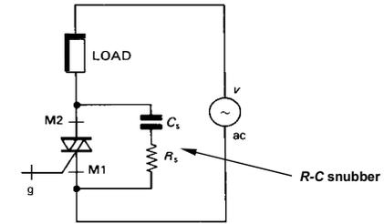
Figure 8.2. Thyristor (triac) ac circuit with an R-C snubber circuit.
