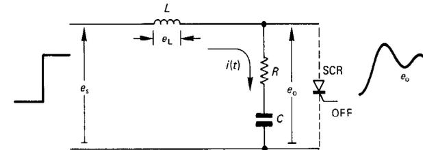
Figure 8.3. Non-polarised R-C snubber equivalent circuit showing the second-order output response eo to a step input voltage es.
