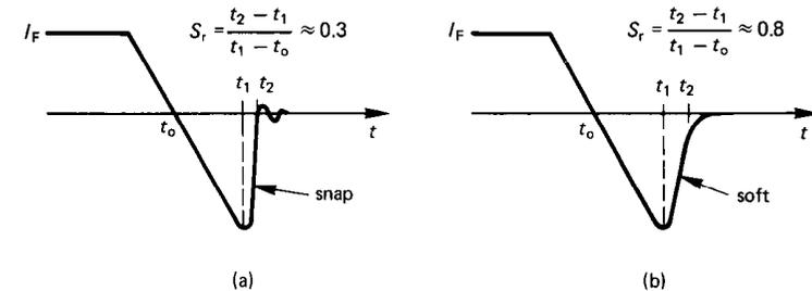
Figure 4.5. Comparison of fast recovery diode  $di_{rr}/dt$  characteristics of:
