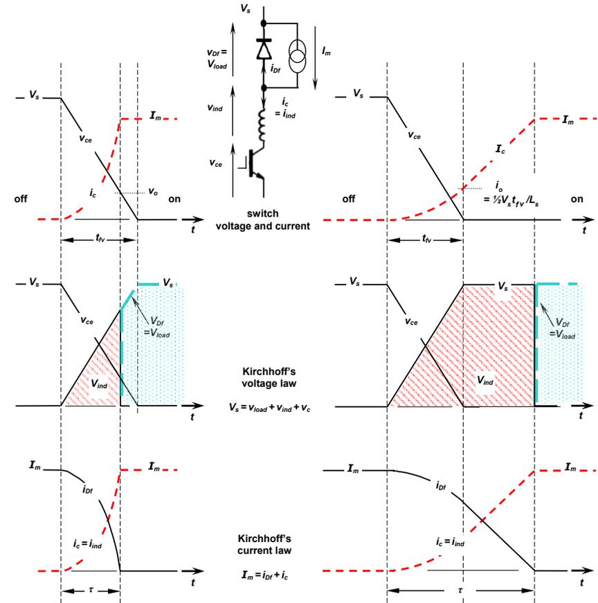
Figure 8.18. Turn-on snubber waveforms satisfying Kirchhoff's laws: (a) turn-on with small snubber inductance and (b) turn-on with large snubber inductance.
