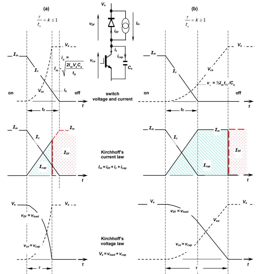
Figure 8.12. Switch turn-off waveforms satisfying Kirchhoff's laws: (a) turn-off with small snubber capacitance and (b) turn-off with large snubber capacitance.
