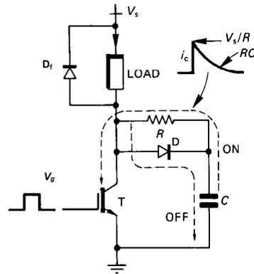
Figure 8.10. Practical capacitive turn-off snubber showing capacitor charging and discharging paths during device switching.
