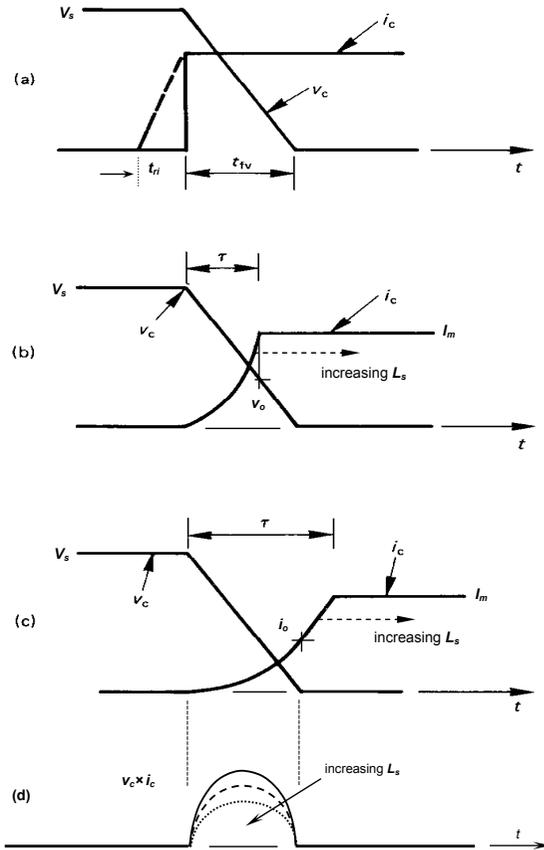
Figure 8.17. Switch voltage and current collector waveforms at turn-on: (a) without a snubber; (b) and (c) with an inductive snubber; and (d) switch power losses.
