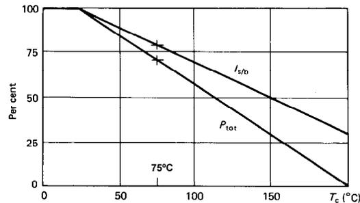
Figure 4.8. Power and second breakdown derating versus case temperature.
