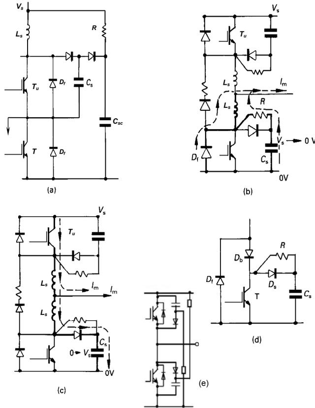
Figure 8.23. Bridge leg configurations: (a) Undeland indirect leg snubber circuit; (b) leg with turn-on snubber and turn-off snubber  $C_s$  discharge path shown; (c) L-C oscillation at switch-on; (d) blocking circuit to prevent snubber capacitor discharge when  $D_i$  conducts; and (e) dual soft voltage clamps for high current single switch modules.
