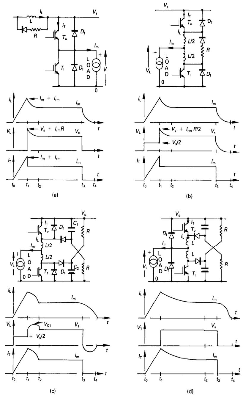
Figure 8.24. Turn-on snubbers for bridge legs: (a) single inductor in dc link; (b) unified L-R-D snubber; (c) soft voltage clamp; and (d) soft voltage clamp with load clamped.
