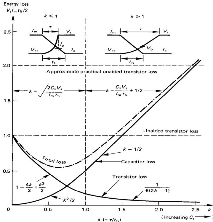
Figure 8.13. Loss components for a switch at turn-off when employing a capacitance-type snubber and assuming the collector current falls according to  $i_c = I_m(1 - t/t_{fi})$ .
