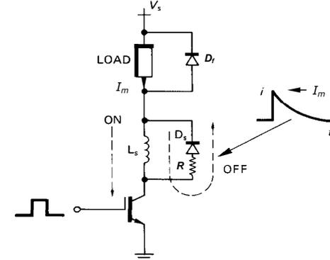
Figure 8.16. Turn-on switching-aid circuit incorporating series inductance,  $L_s$ .
