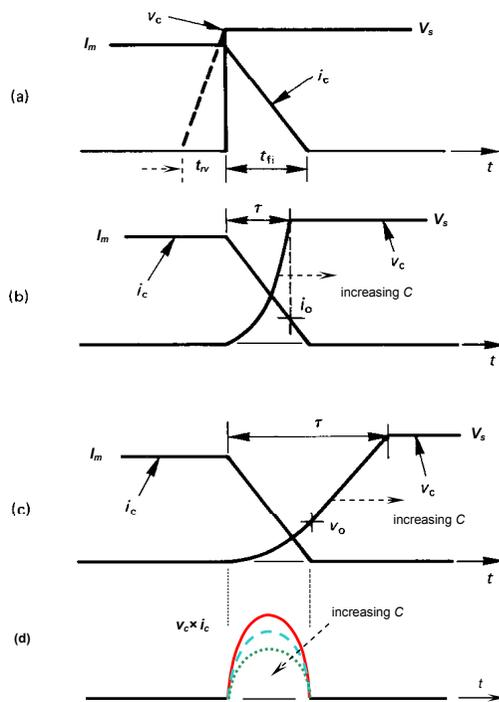
Figure 8.11. Switch turn-off waveforms: (a) unaided turn-off; (b) turn off with small snubber capacitance; (c) turn-off with large snubber capacitance; (d) and switch power losses.
