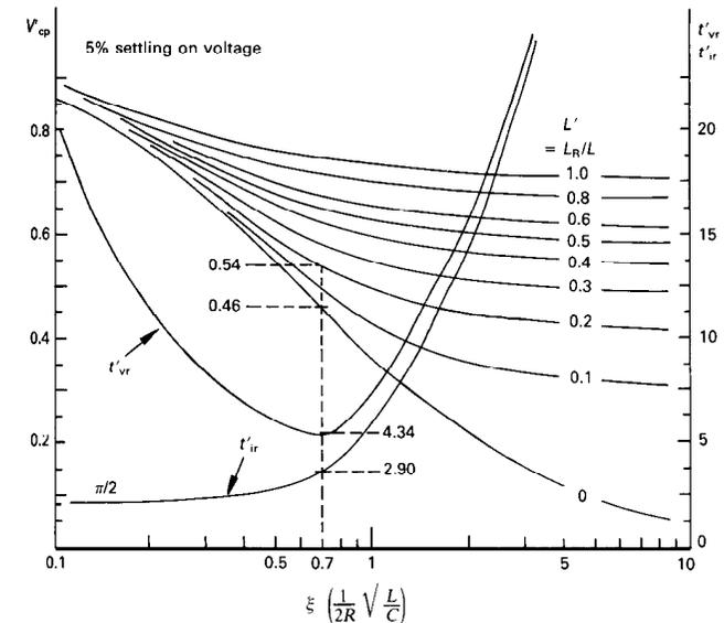
Figure 8.7. Voltage clamp capacitor normalised peak over-voltage,  $V_{cp}'$ , versus damping factor,  $\xi$ , for different resistor normalised inductances,  $L'$ , and voltage and current normalised settling times,  $t_{vr}'$ ,  $t_{vr}' = V_{cp}' / \{I_m \sqrt{L/C}\}$ ,  $t_{vr}' = t_{vr} / \omega_0$ ,  $t_{ir}' = t_{ir} / \omega_0$ .
