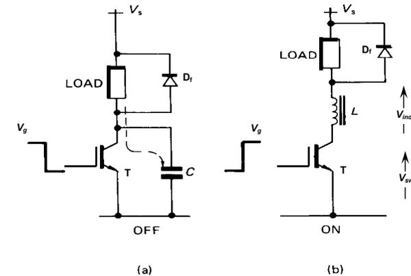
Figure 8.9. Basic switching-aid circuits comprising: (a) a parallel capacitor for current shunting at switch turn-off and (b) a series inductor for supporting voltage, thus limiting the rate of rise of principal current at turn-on.
