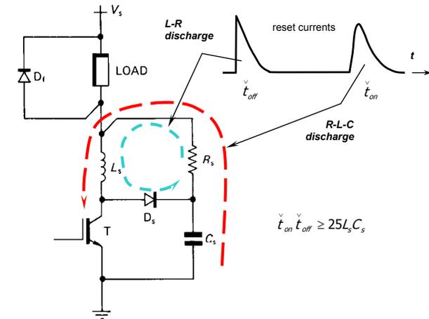
Figure 8.22. Unified snubber incorporating both a turn-on and a turn-off circuit which share the one dissipation reset resistor.
