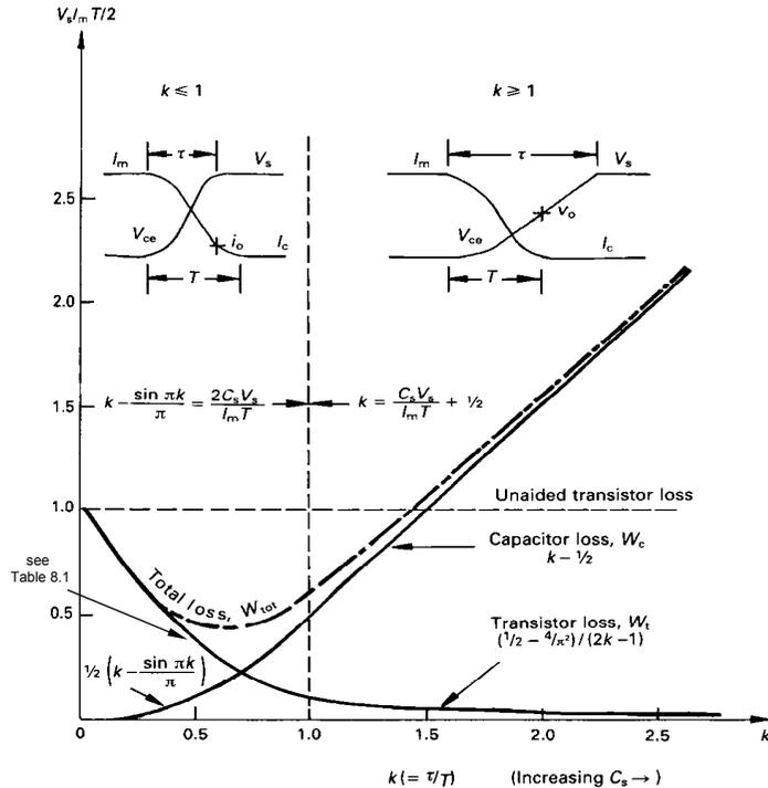
Figure 8.15. Loss components for a switch at switch-off when employing a capacitance-type snubber and assuming a collector fall current according to  $i_c = \frac{1}{2} I_m \{1 + \cos(\pi t/T)\}$ .
