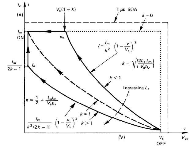
Figure 8.20. The collector  $I$ - $V$  trajectory at turn-on with a switching-aid circuit.
