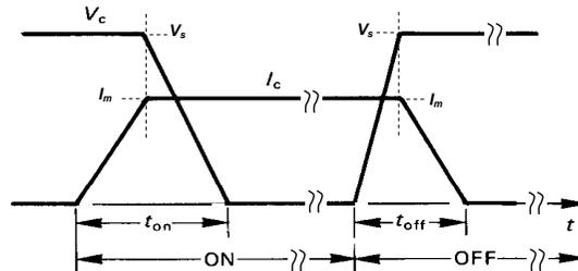
Figure 8.8. Idealised collector (anode) switching waveforms for an inductive load.
