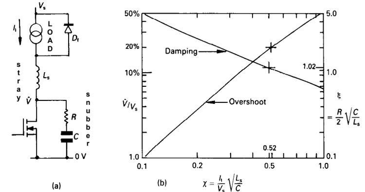
Figure 8.1. MOSFET drain to source  $R$ - $C$  snubber protection: (a) MOSFET circuit showing stray inductance,  $L_s$ , and  $R$ - $C$  protection circuit and (b)  $R$ - $C$  snubber optimal design curves.
