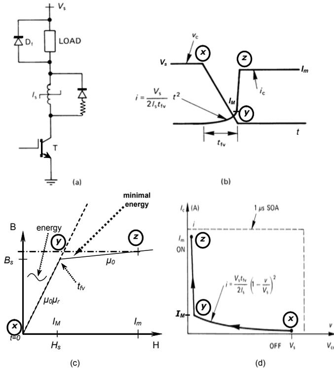
Figure 8.21. Switch turn-on characteristics when a saturable inductor is used in the turn-on snubber: (a) circuit diagram; (b) collector voltage and current waveforms; (c) magnetic core  $B$ - $H$  curve trajectory; and (d) safe operating area  $I$ - $V$  turn-on trajectory.
