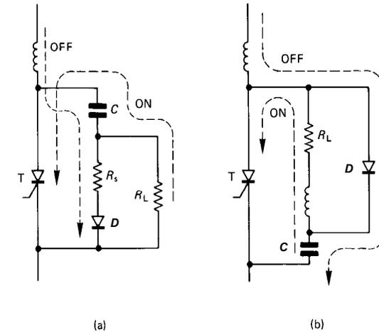
Figure 8.5. Polarised variations of the basic thyristor R-C snubber: (a)  $R_s \ll R_L$  and (b) transistor-type R-C-D snubber,  $R_s = 0$ .
