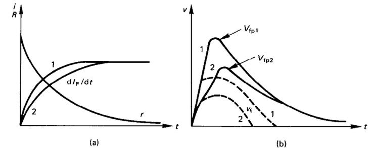
Figure 4.3. Diode forward turn-on characteristics for two initial anode  $di/dt$  cases:
